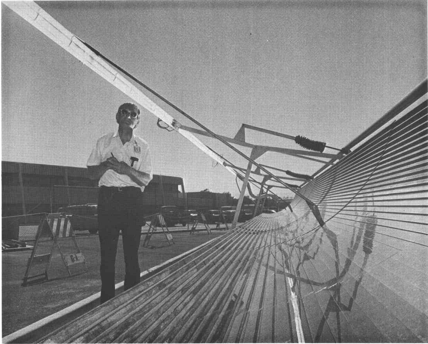
Fig. 4. Heat receiver under test
