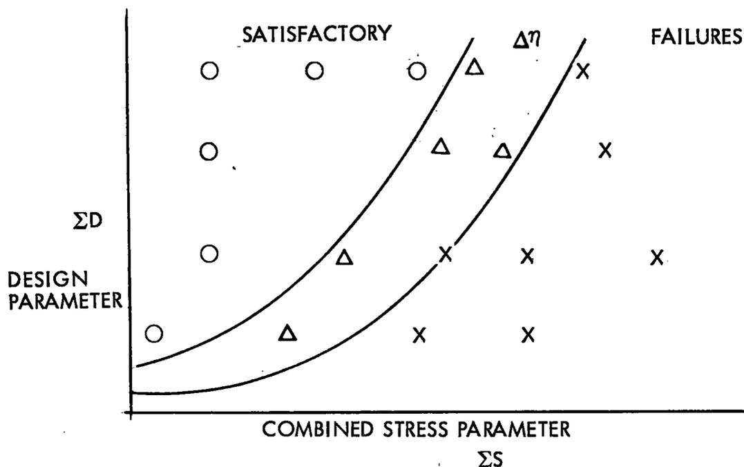
Figure 13. Failure envelope defined by testing various combinations of design and stress parameters.
