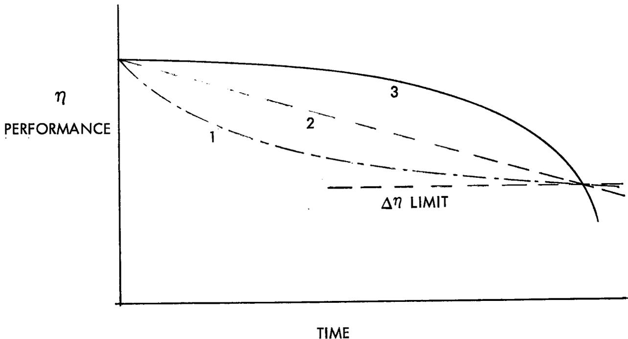
Figure 14. Typical performance degradation curves determined by differing aging and degradation mechanisms.
