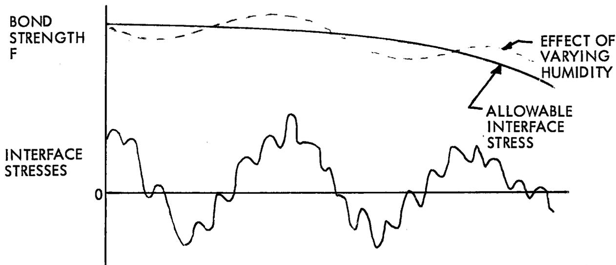
Figure 9. Allowable interface stresses and applied stresses due to outdoor exposure of encapsulated module.
