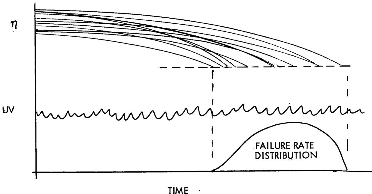
Figure 6. Failure rate distribution due to variable stress and variable design parameters.
