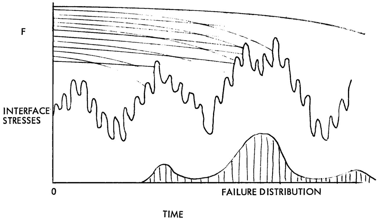
Figure 10. Failure rate distribution due to the interaction of several aging modules with time varying applied stresses.
