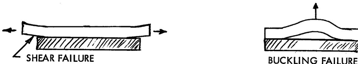
Figure 8. Two types of delamination failure due to differential expansion strains.
