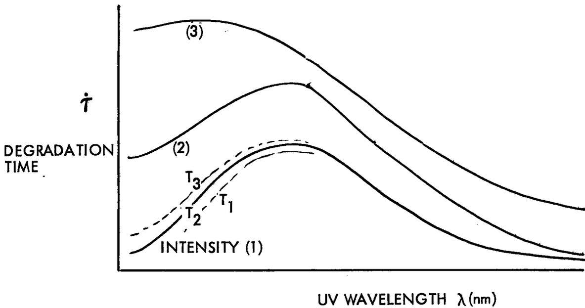
Figure 4b. Rate of degradation of cover material exposed to UV.
