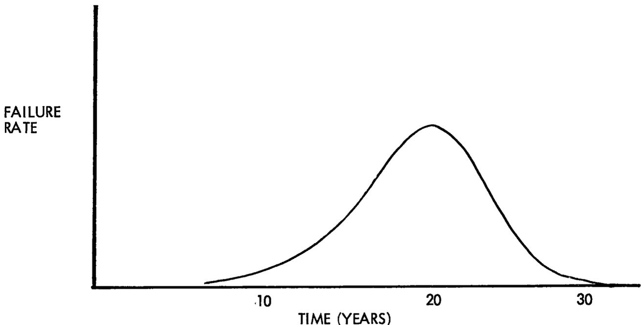
Figure 1. Failure rate distribution for solar array modules.
