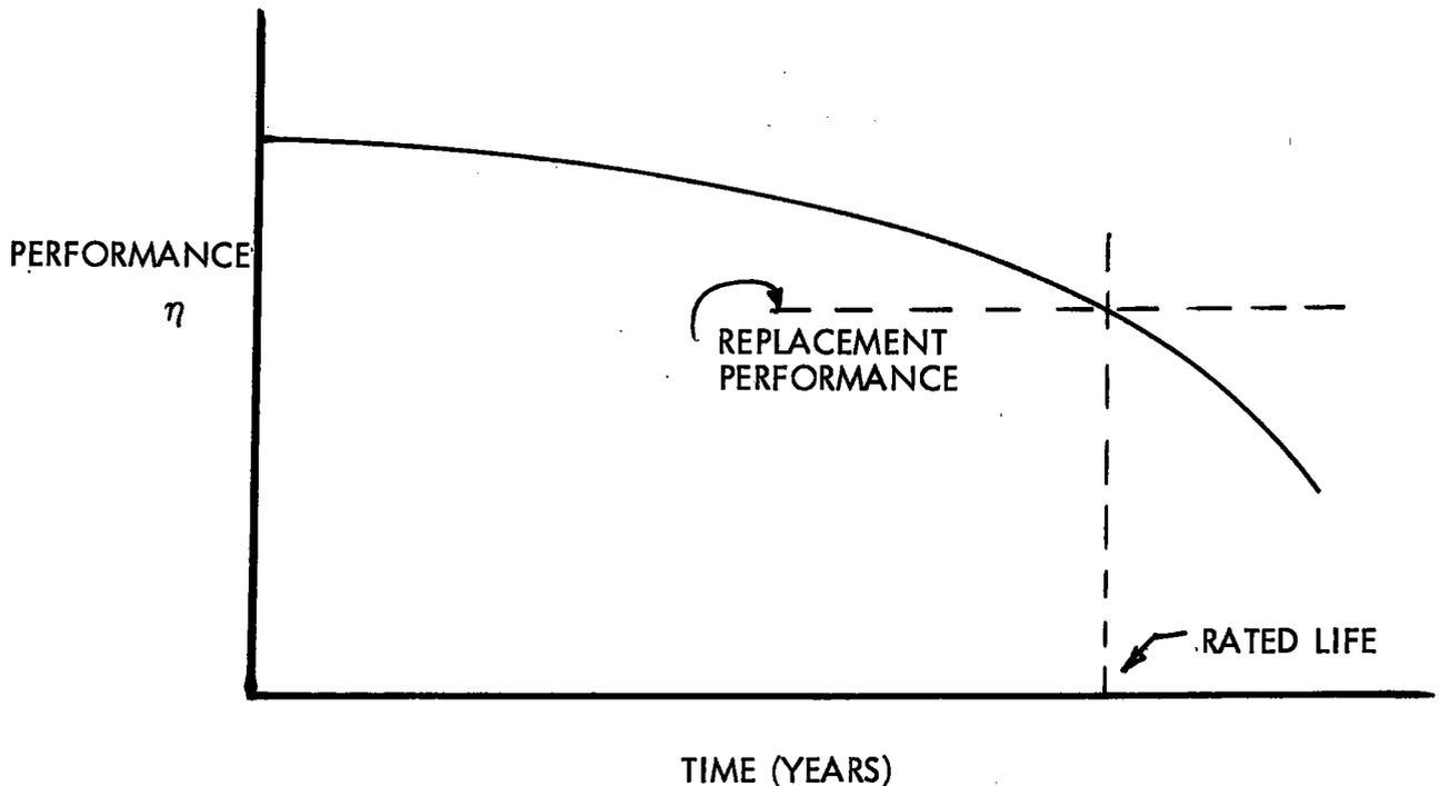
Figure 2. Solar module life time performances due to UV degradation of cover material.
