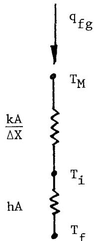
$q_{fg}$  = Incoming flux, measured value from flux gage measurement,
