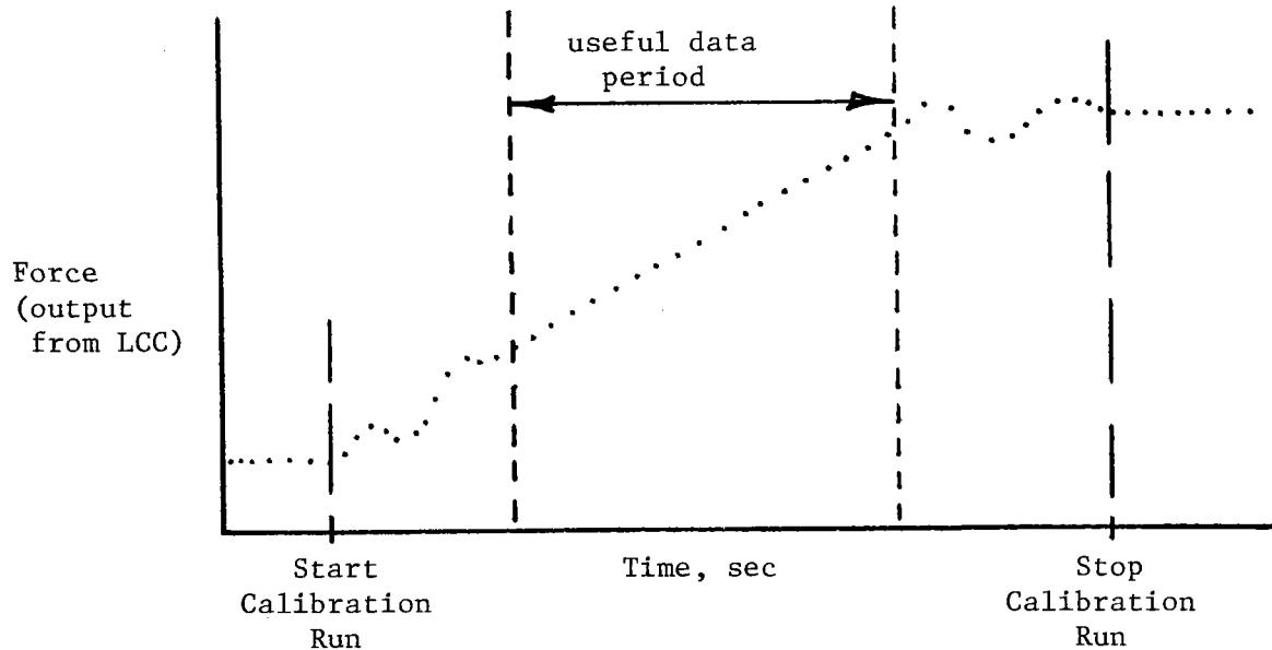
The problem is to identify the "useful data period" during the calibration run and then to fit a linear curve (Force vs time) to the points within the "useful data period." The slope of this curve, expressed in lbm/hr, is the quantity we are seeking.
