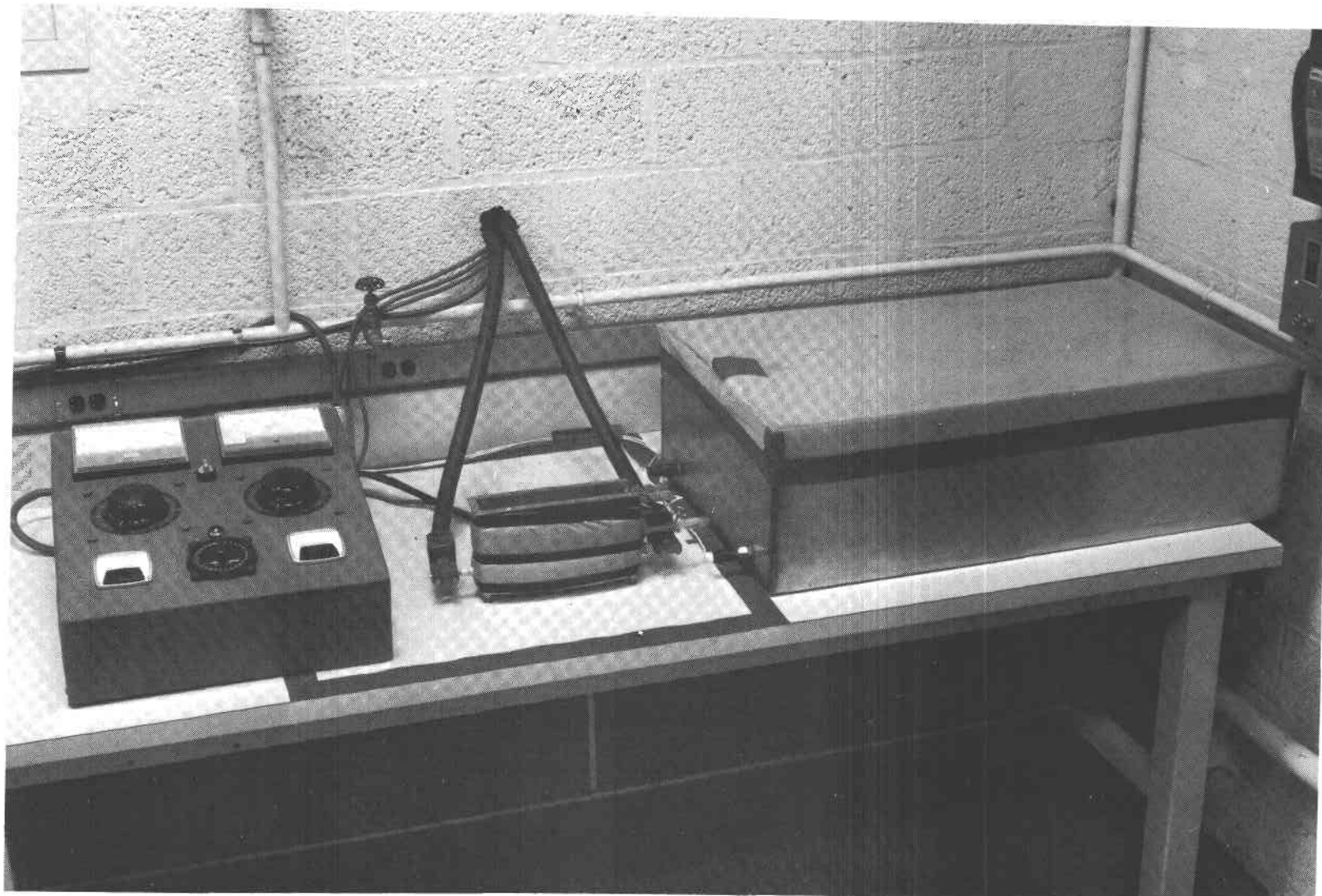
Figure 8 4 Wick Boiling Experimental Test Setup Showing Control Panel, Primary Tank, and Secondary Tank
