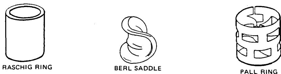
FIGURE A.1. Typical Packings for a Direct-Contact Molten Salt Heat Exchanger
