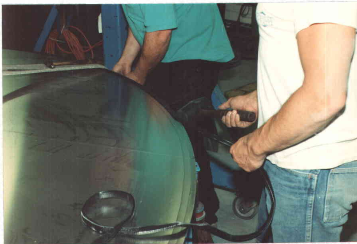
Installing edge protection molding. To protect against cuts, the rough edges of the membranes are covered with an edge molding on the front and back edges of the facet.
