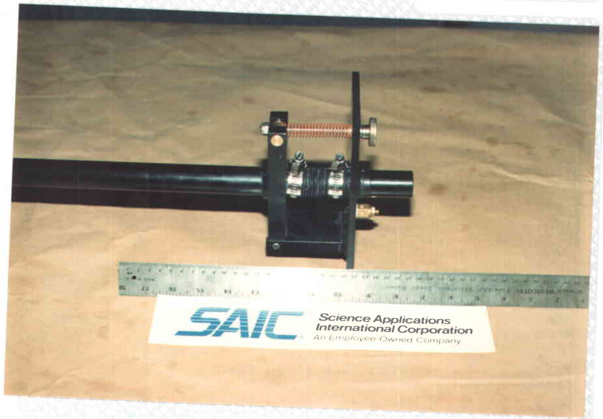
Facet focus control focus adjustment assembly. The completely assembled facet focus control assembly.
