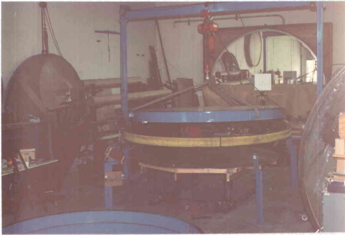
Removing completed facet from tensioning ring. The completed facet is disengaged from its mounts and lifted from the tensioning ring.
