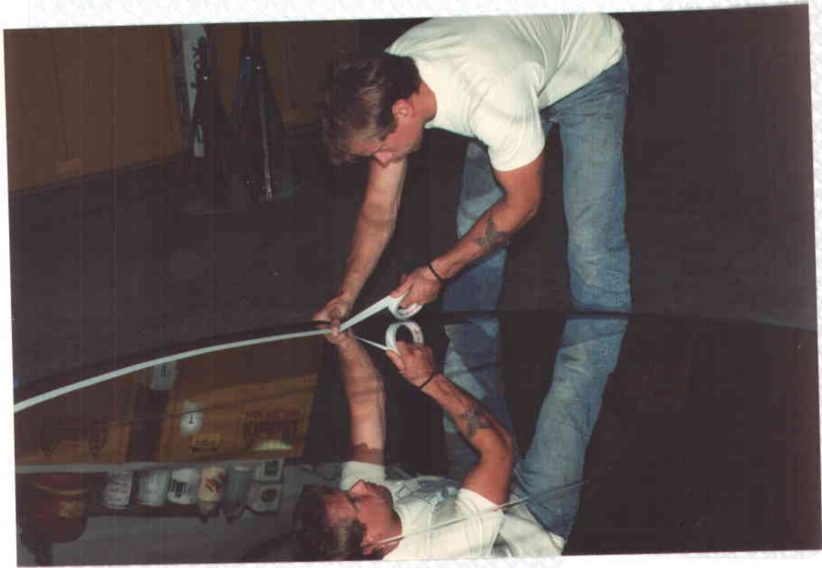
Taping edge of reflective film with Tedlar™ tape. Tedlar™ tape is applied around the periphery of the reflective film in order to weather seal that area.
