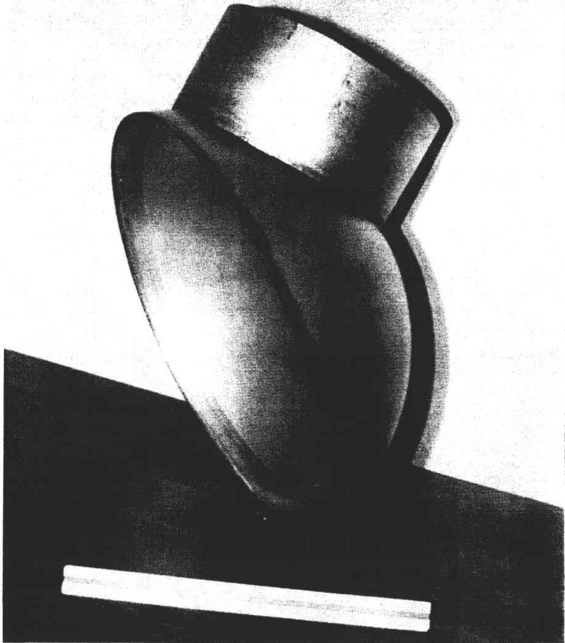
Figure 4. First pair of domes and section of condenser welded together to verify manufacturing processes for pool-boiler receiver.
