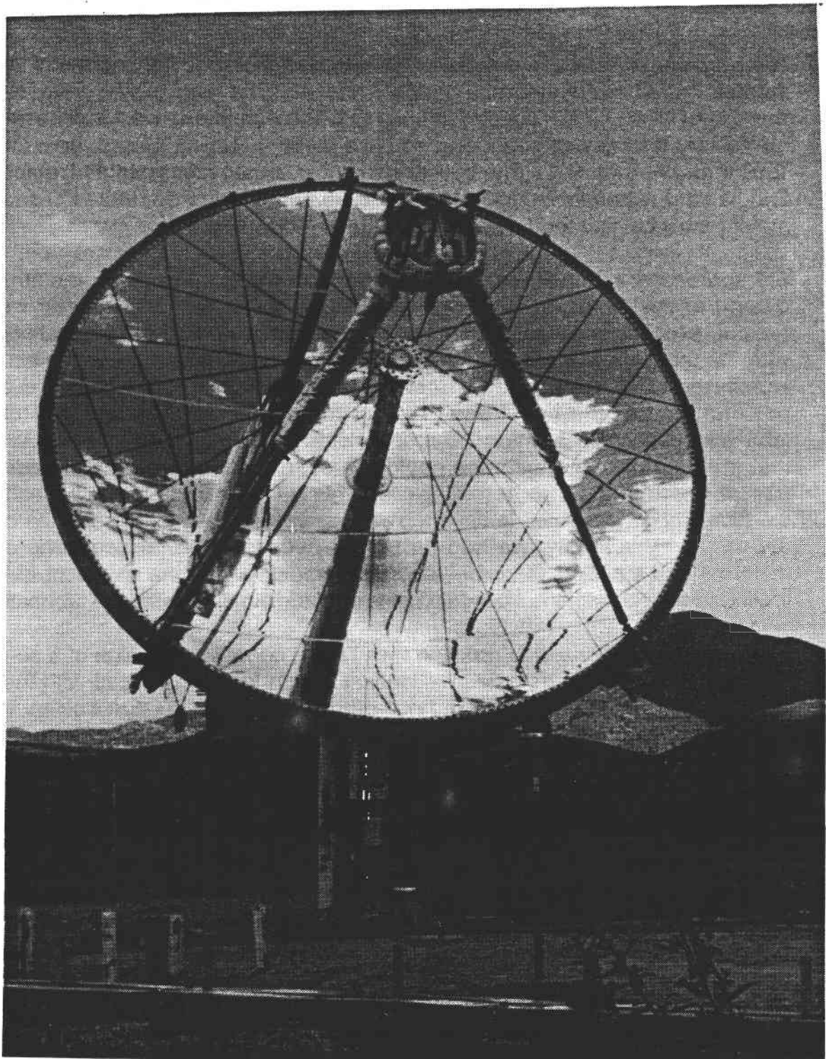
Figure 2.B.1 The 7-meter diameter stretched-membrane concentrator on test at Sandia's National Solar Thermal Test Facility in Albuquerque, NM.
