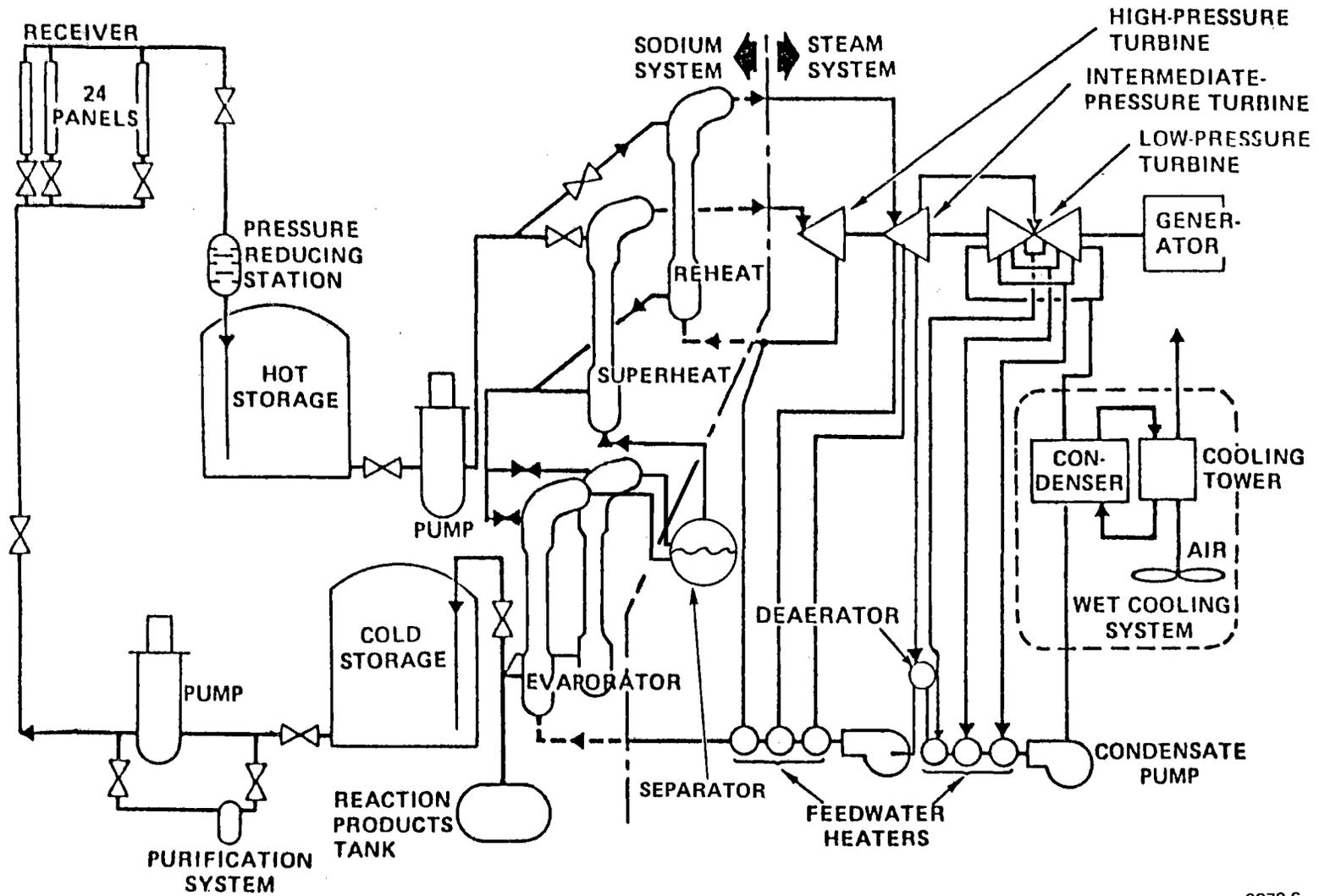
Figure 15. Advanced Central Receiver System
