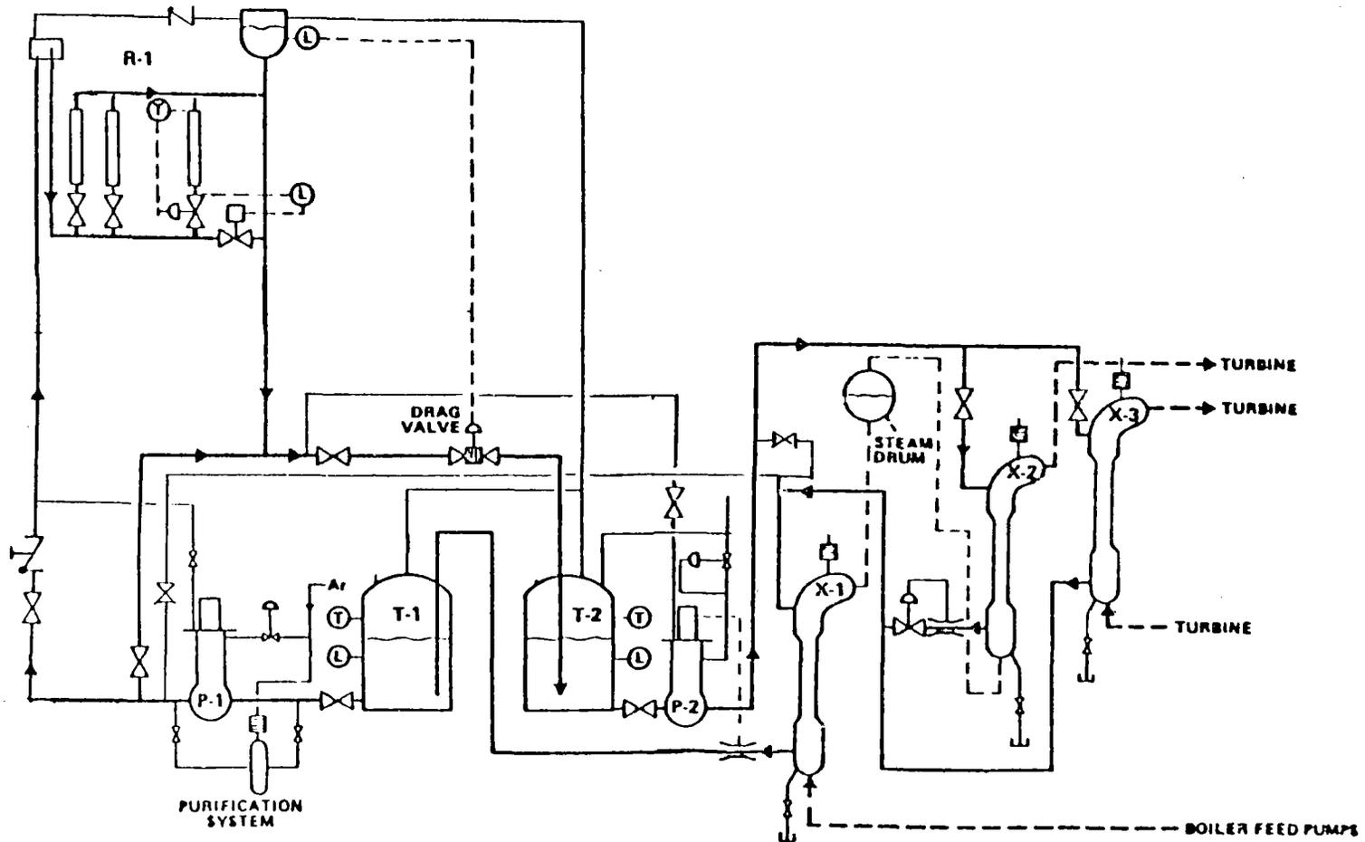
Figure 6. Sodium Heat Transport System
