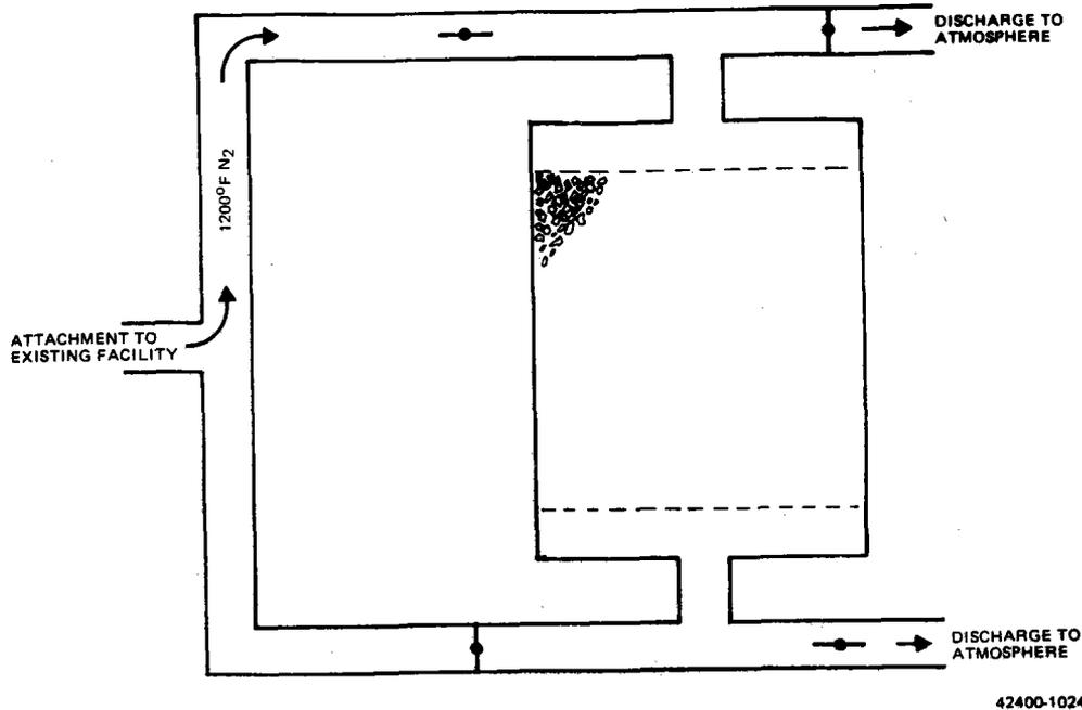
b. Schematic of Air-Rock Thermocline Test
