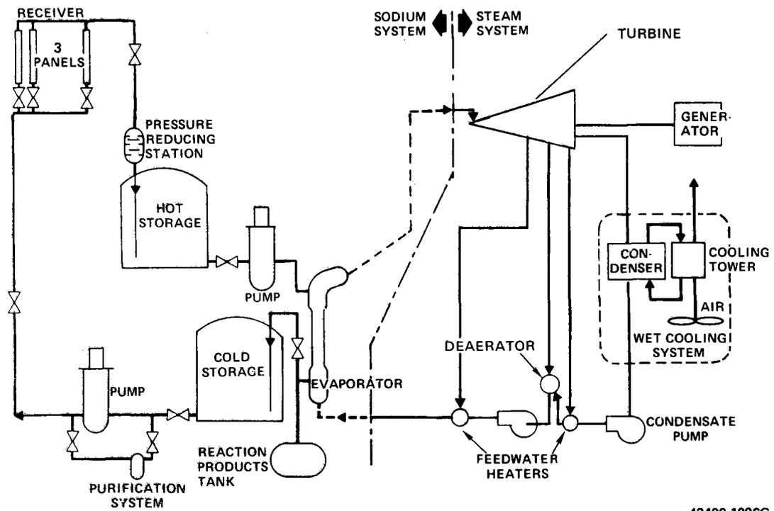
Figure 3. Advanced Central Receiver System (10-MWe Pilot Plant)
