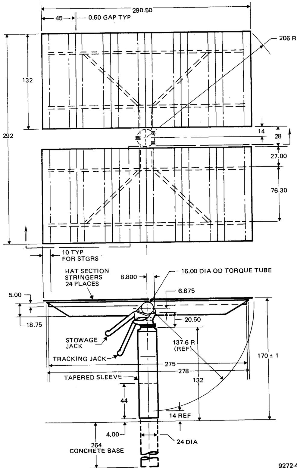
Figure 11. Heliostat Assembly
