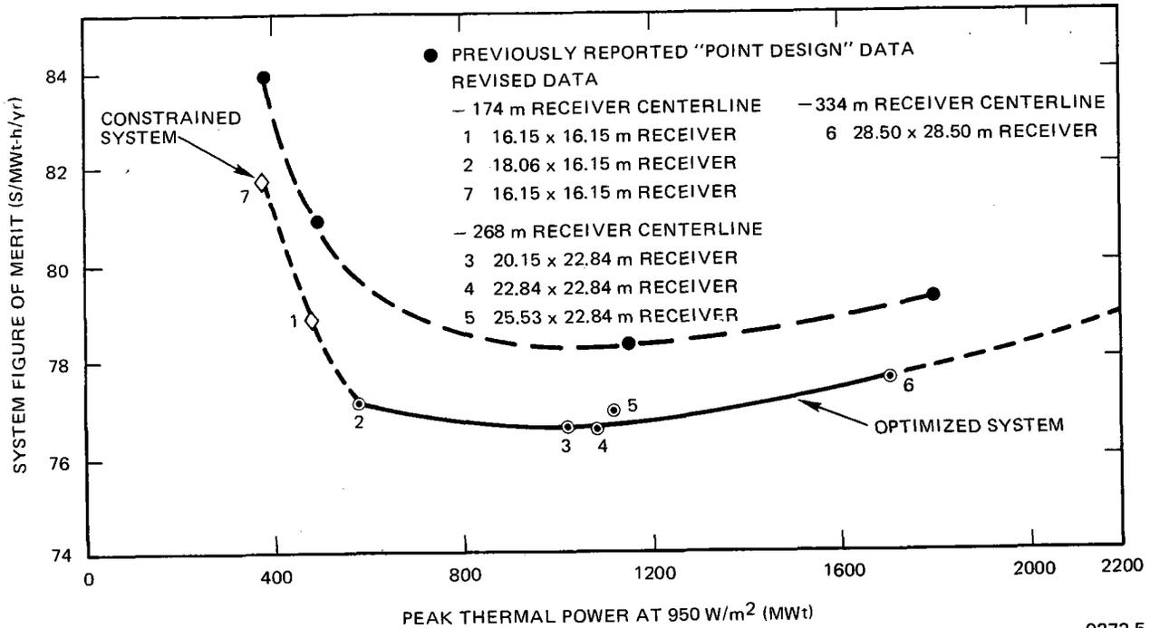
Figure 14. Expanded Thermal Capacity Optimization Analysis Results
