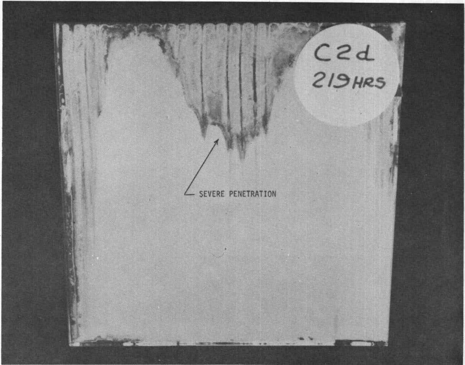
Figure D-5 Salt Spray Coupon C2d Laminated with Cut Edge
