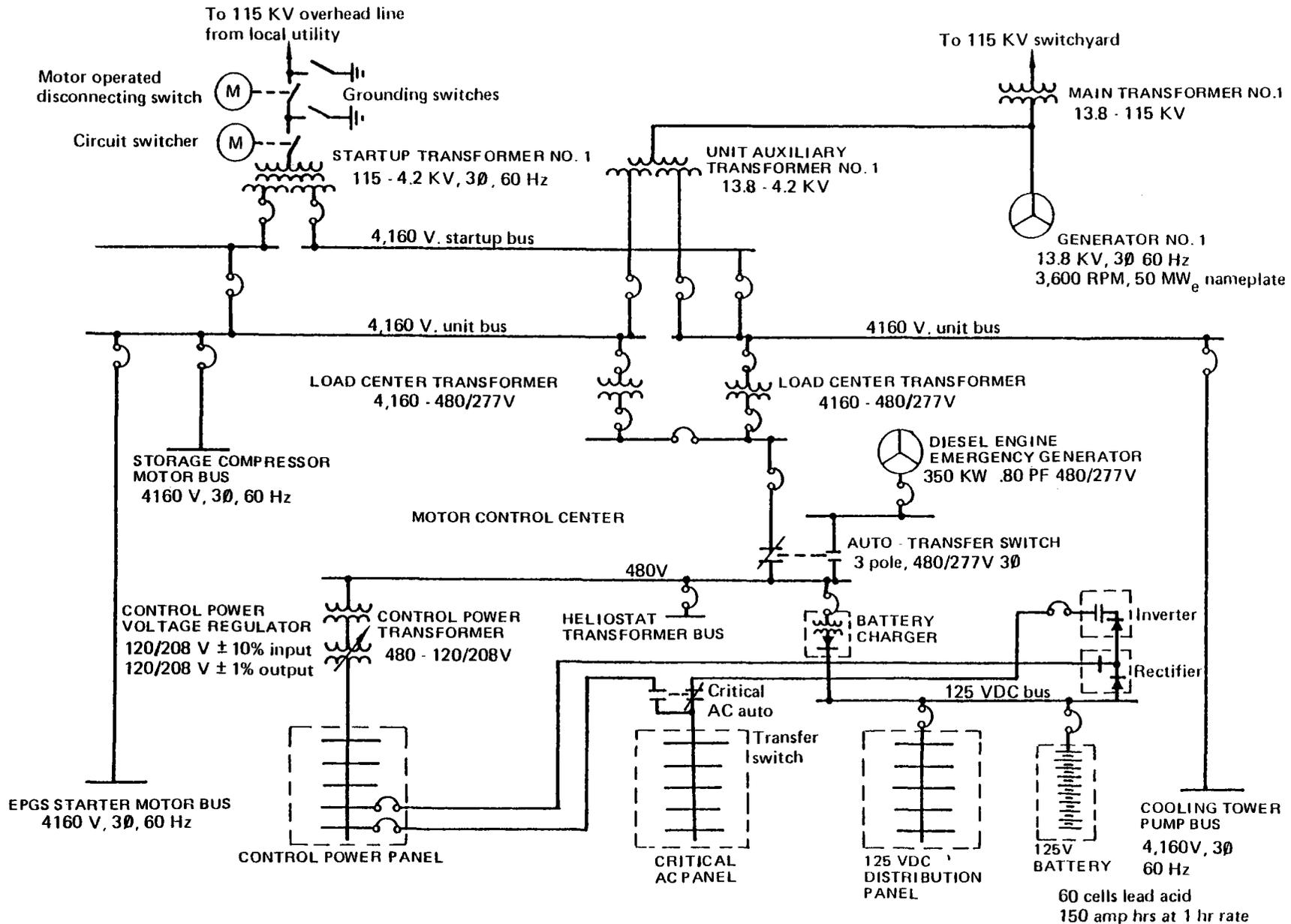
Figure 3.3.1-8. Single Line Plant Power Schematic
