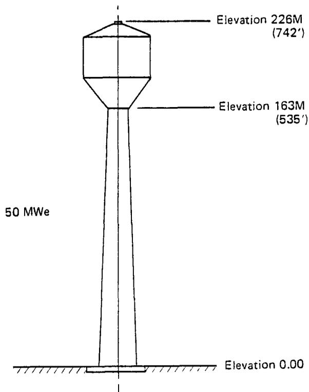
Figure 3.3.1-1. Receiver Tower Geometry - 50 MW<sub>E</sub> Critical Module
