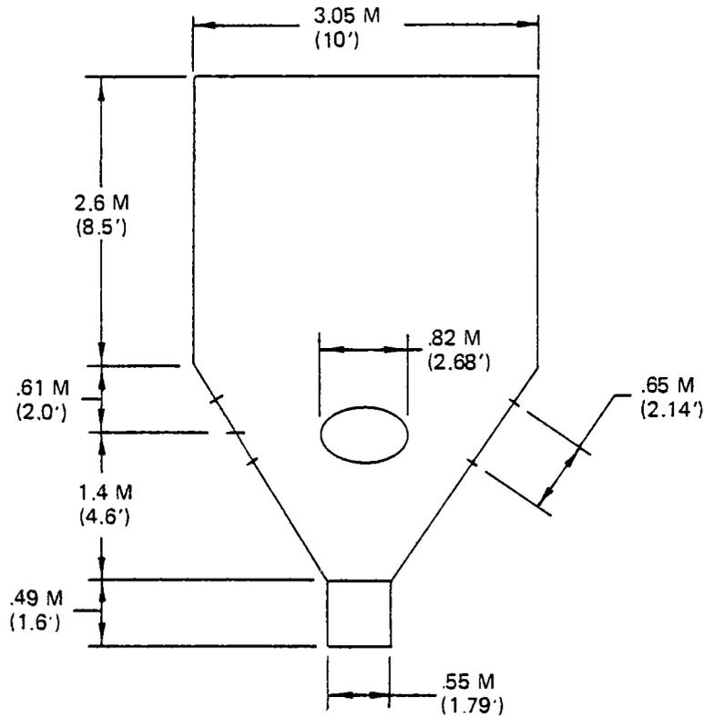
Figure 4.1.3.1-1. Model Receiver for Convective Loss Test
