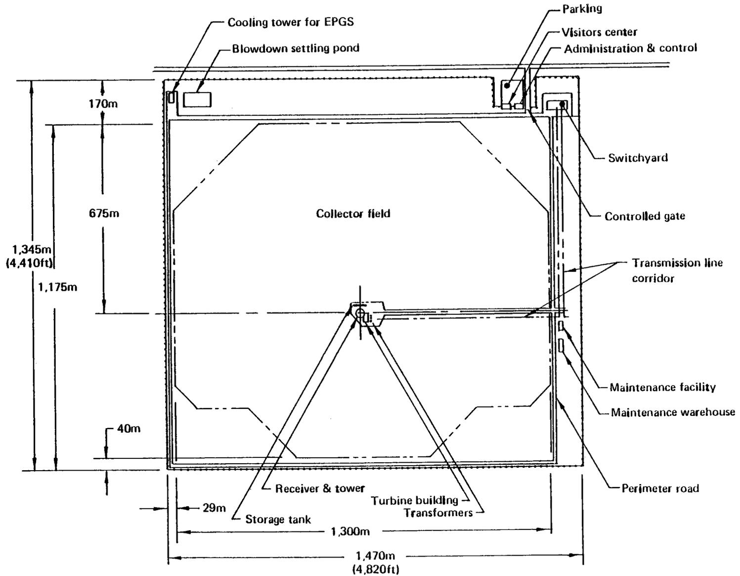
Figure 3.3.1-5. Plant Layout 50 MW<sub>e</sub> Critical Module
