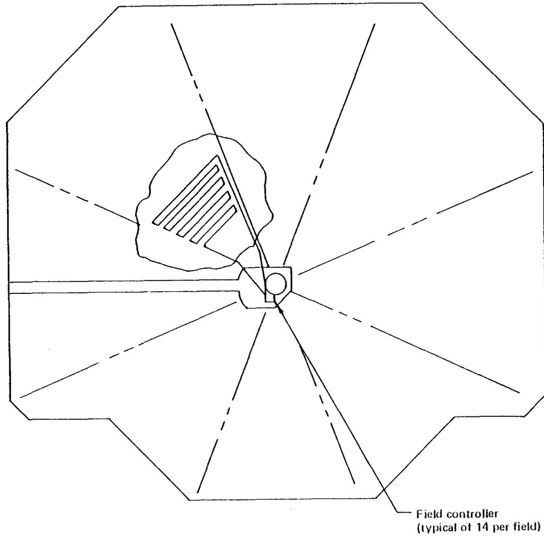
Figure 3.3.1-7. Collector Field Control Cable Layout
