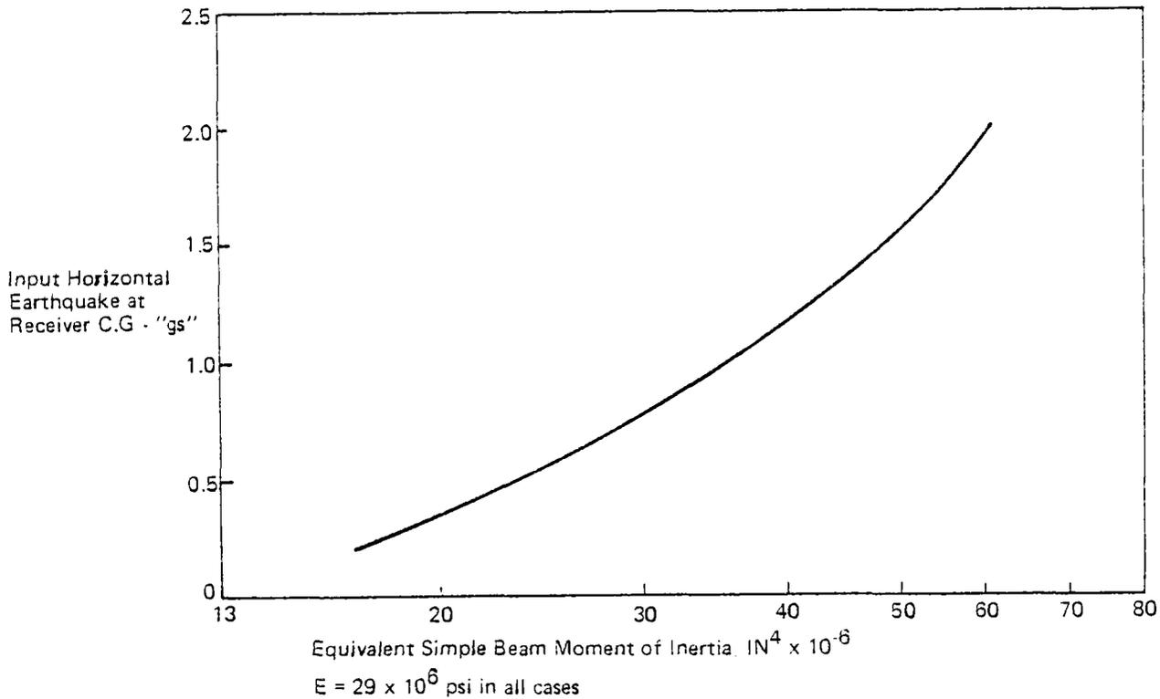
Figure 3.3.1-3. Receiver Elasticity
