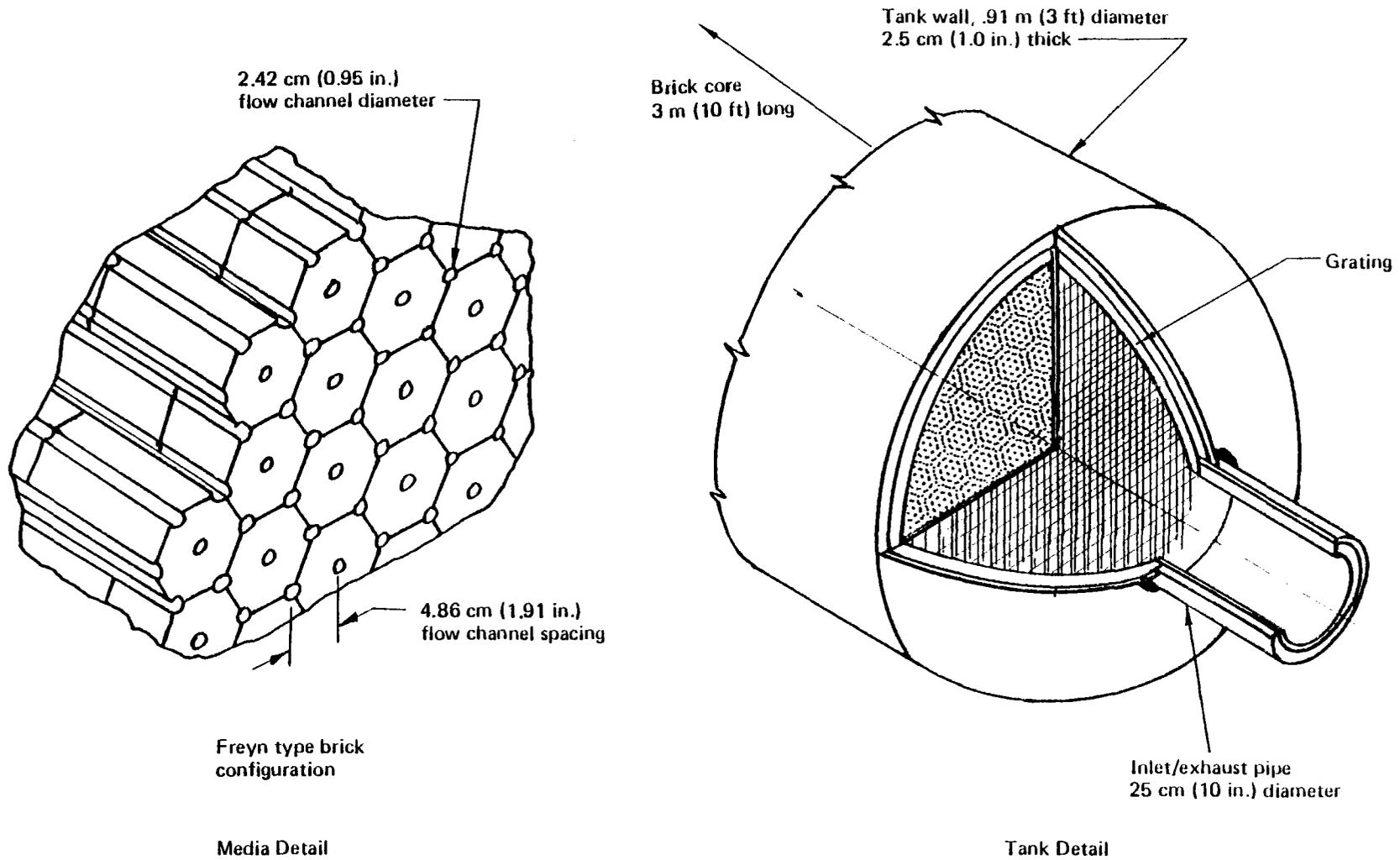
Figure 4.2.3.1-1. Sensible Heat Storage SRE Model Configuration
