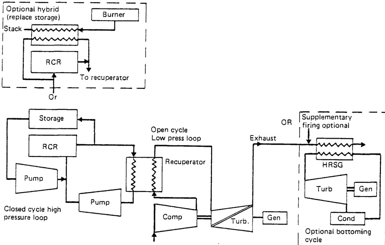
Figure 2.6-1. Dual Loop Solar Plant with Options
