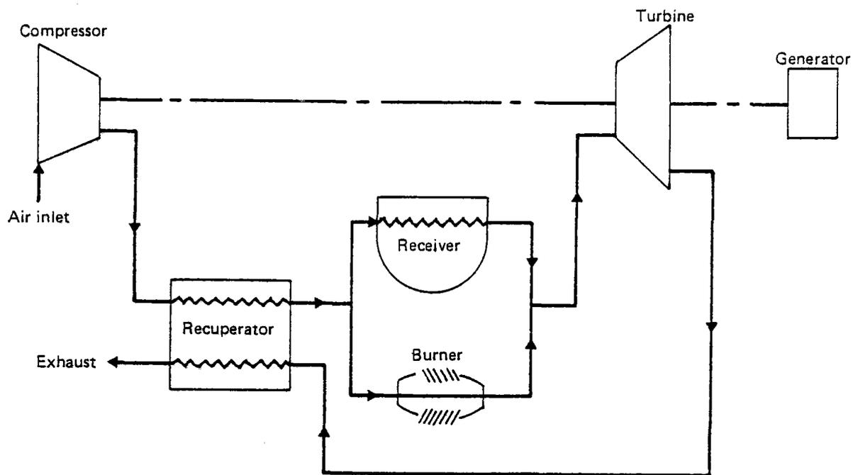
Figure 3.2.1.3-1. EPRI Experimental Plant System Schematic
