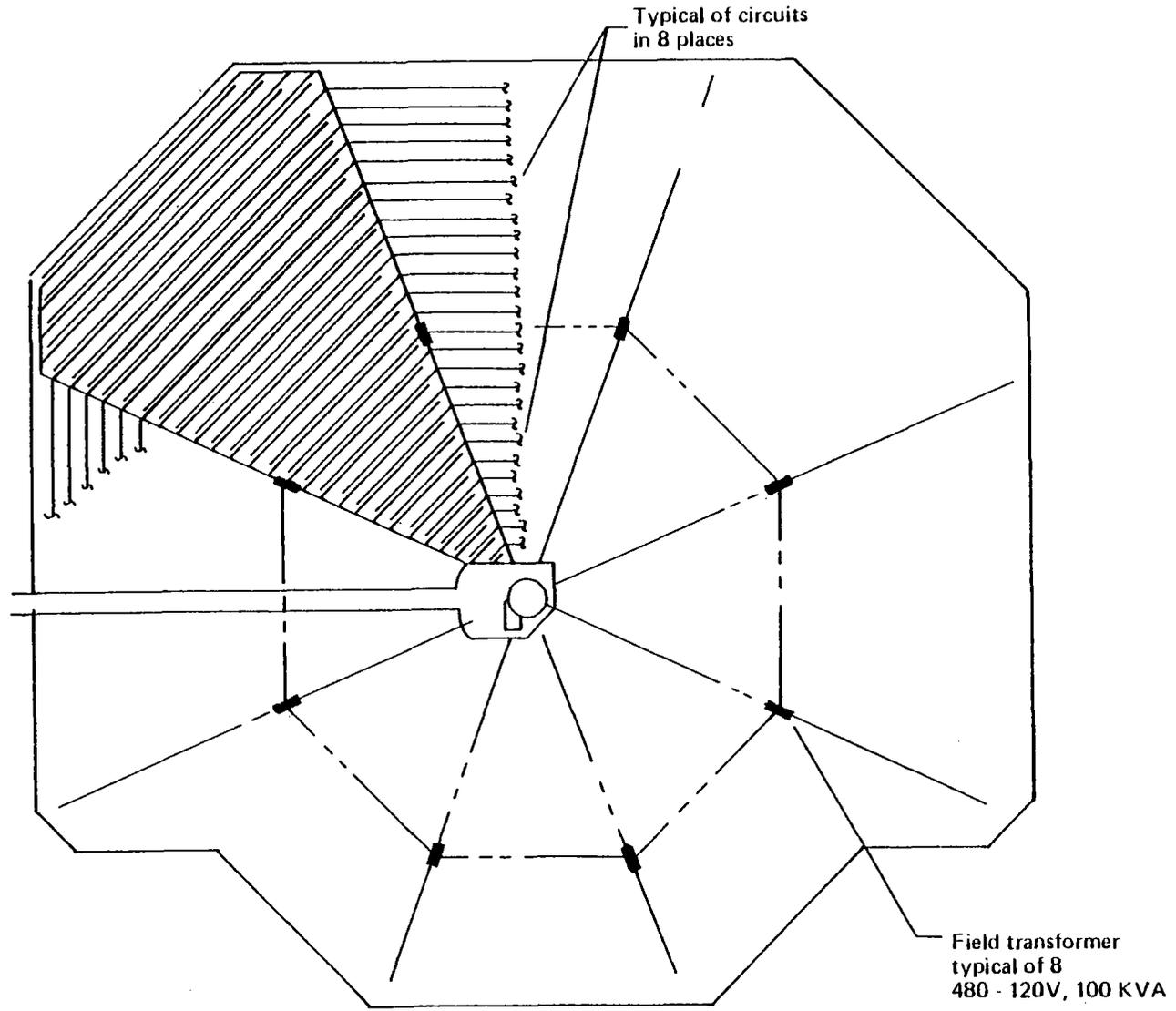
Figure 3.3.1-9. Single Line Field Power Arrangement
