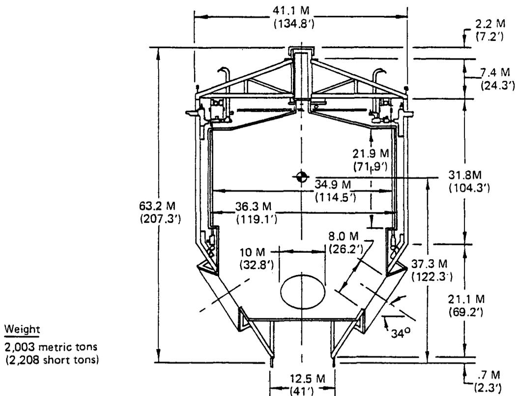
Figure 3.3.1-2. Critical Module Receiver Configuration
