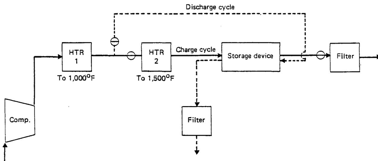
Figure 4.2.3.3-1. Sensible Heat Storage SRE Charge and Discharge Simulator
