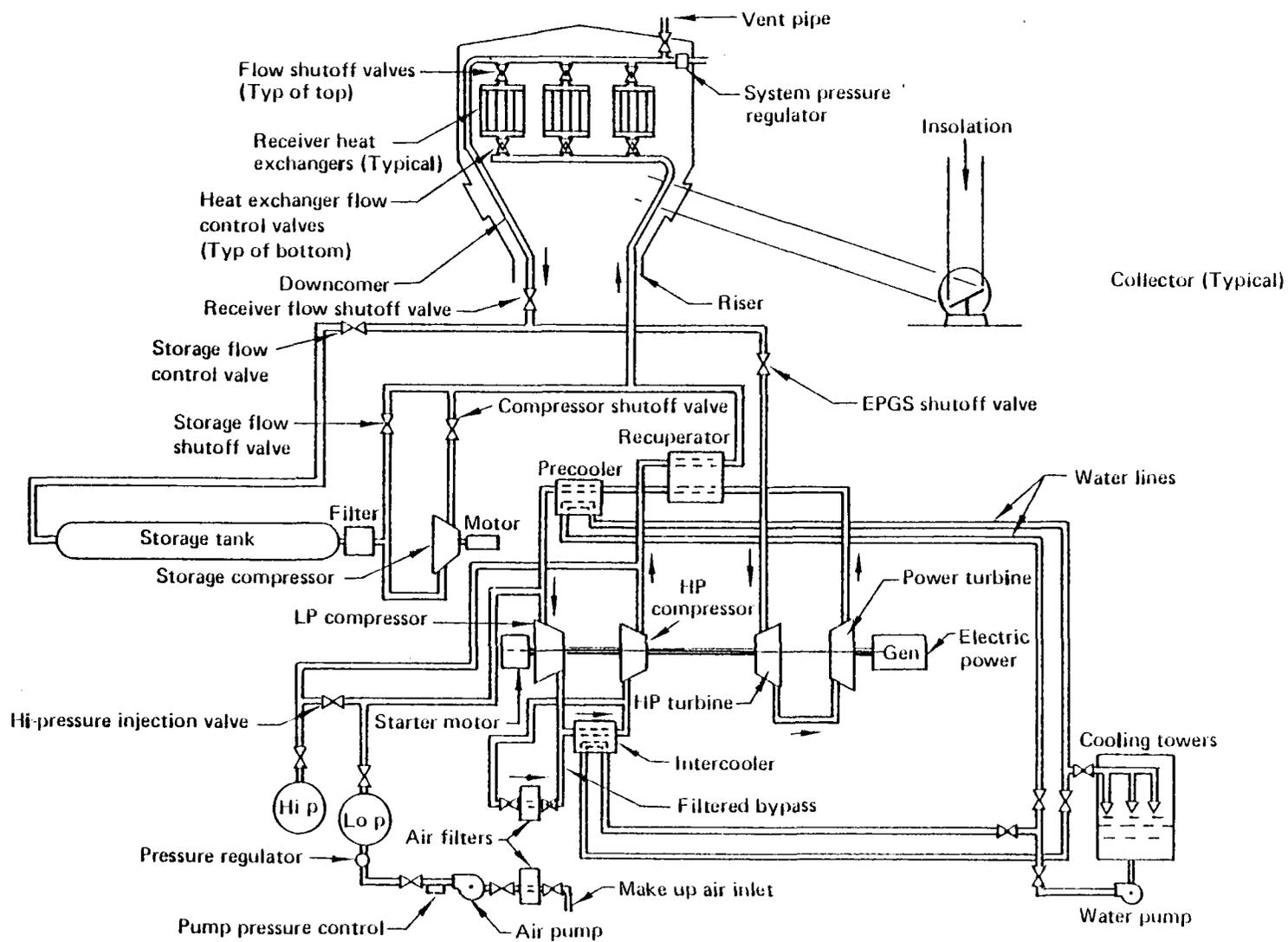
Figure 3.3.1-6. 50 MWe ACR Solar Power System Schematic
