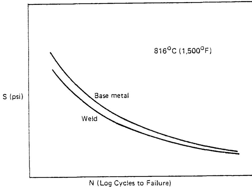
Figure 4.1.1.2-1. Material Fatigue Characterization
