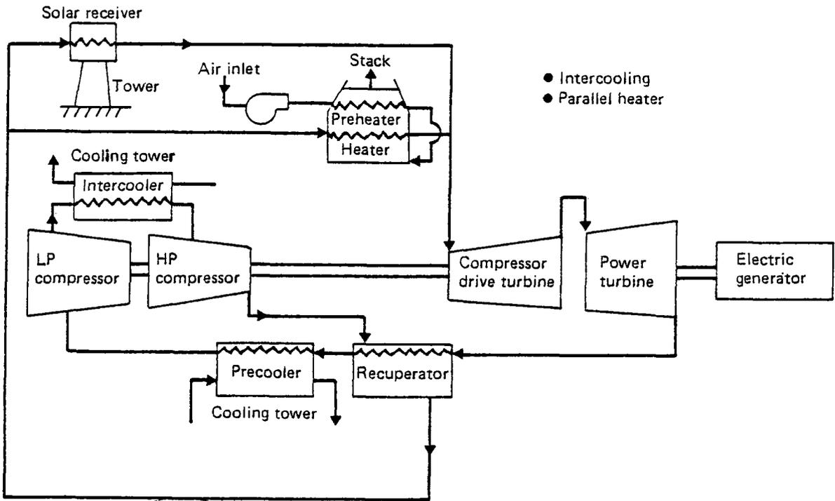
Figure A-2. Baseline Solar Hybrid Power Conversion System
