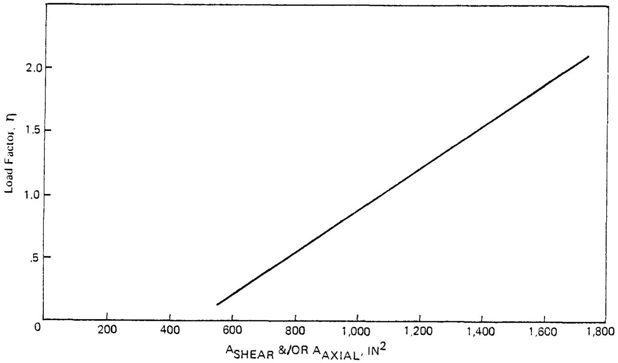
Figure 3.3.1-4. 50 MW<sub>e</sub> Receiver Load Factors
