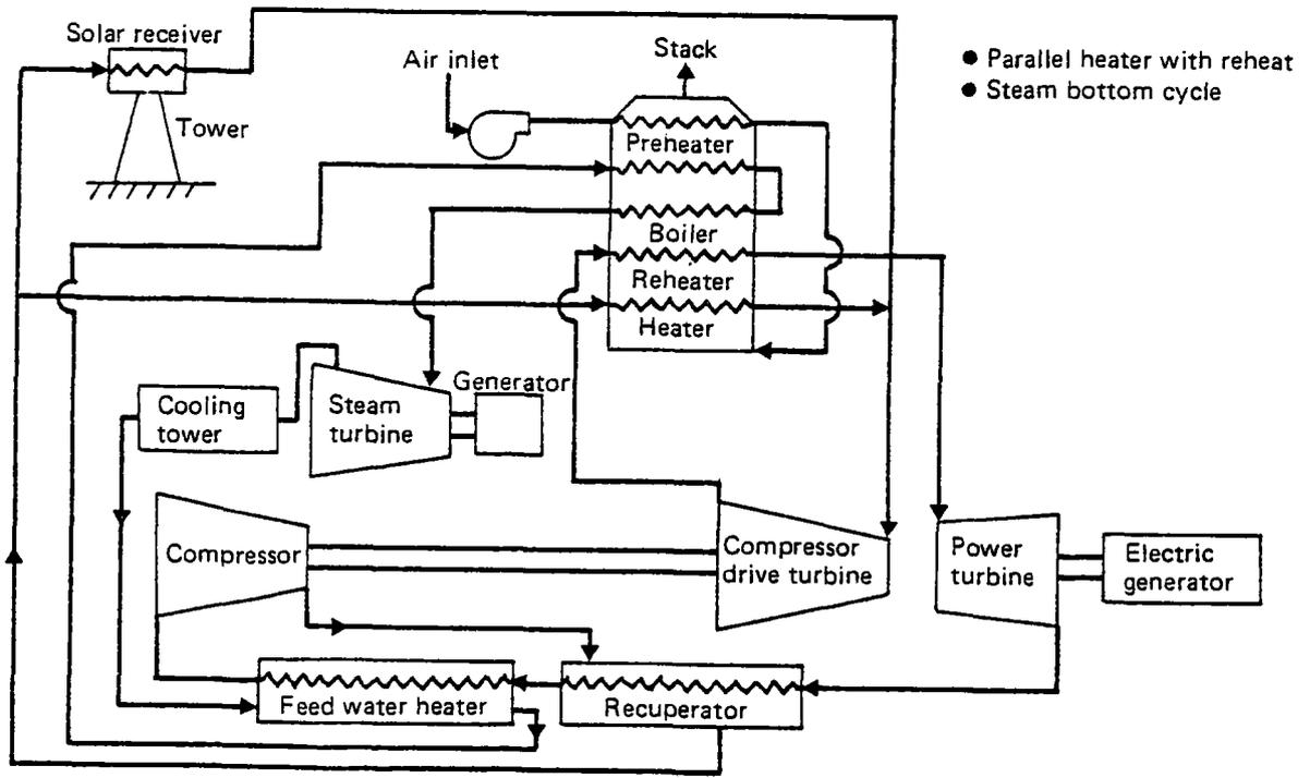
Figure A-3. Closed Brayton Cycle/Steam Combined Cycle Concept
