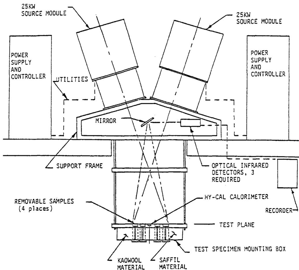
Figure 4.1.2-2. Long Term Exposure Insulation Test Schematic-High Flux Test Facility
