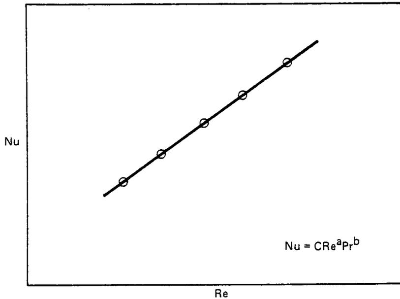
Figure 4.1.3.3-1. Convection Loss Scaling Relationship
