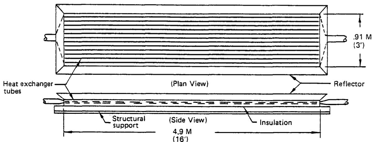
Figure 4.2.1.1-1. Heat Exchanger Panel Configuration
