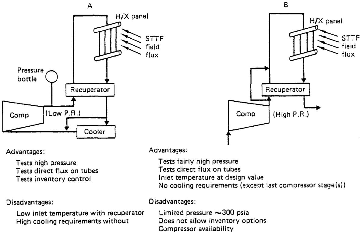
Figure 3.1.2-1. Heat Exchanger Panel Critical Experiment Options
