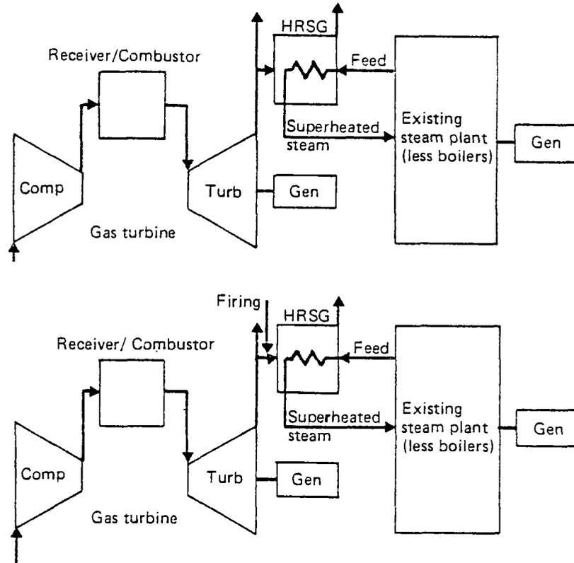
Figure A-1. Unfired and Supplementary-Fired Open Brayton/ Steam Combined Cycle Plants
