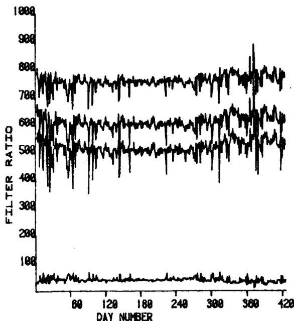
Daily filter ratios, top to bottom, OG1/WG7, RG2/WG7, RG8/WG7, and UV/WG7 for 1-79 thru 2-80 (1000 = 1.000 WG7).
