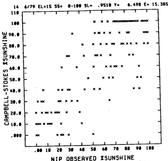
Fig. 8. Hourly Percent Sunshine from Campbell-Stokes Recorder Versus Percent Sunshine from Pyrheliometer (Threshold 200 W/m<sup>2</sup>) for June 1979.
