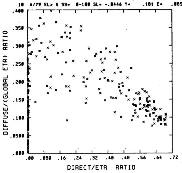
Fig. 9. Hourly Diffuse/(Extraterrestrial on Horizontal Surface) versus Direct/Extraterrestrial for April 1979.
