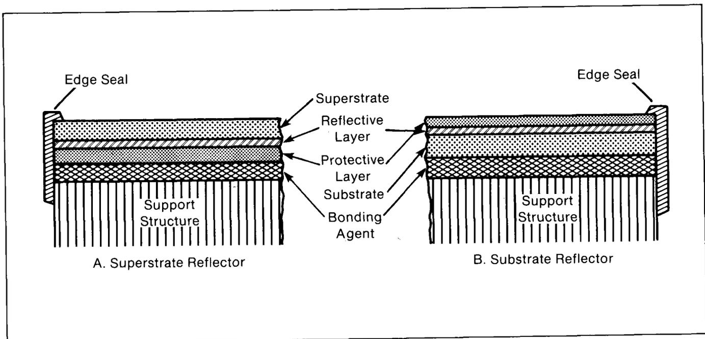
Figure 2-12 Examples of Typical Reflective Surfaces (Bouquet 1980)
