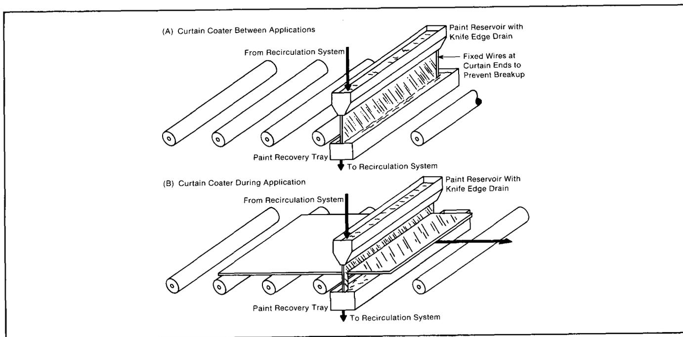
Figure 5-8 Curtain-Coater Operation: (A) Between Applications, and (B) During Application (Lind et al. 1979)
