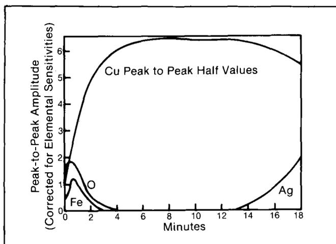
**Figure 3-4a Auger Electron Depth Profile Through the Copper Layer of a One Year Old Mirror after Removal of a Lacquer Backing with Acetone.** The profile has been corrected for elemental sensitivity factors as provided by Physical Electronics (Thomas 1983)
