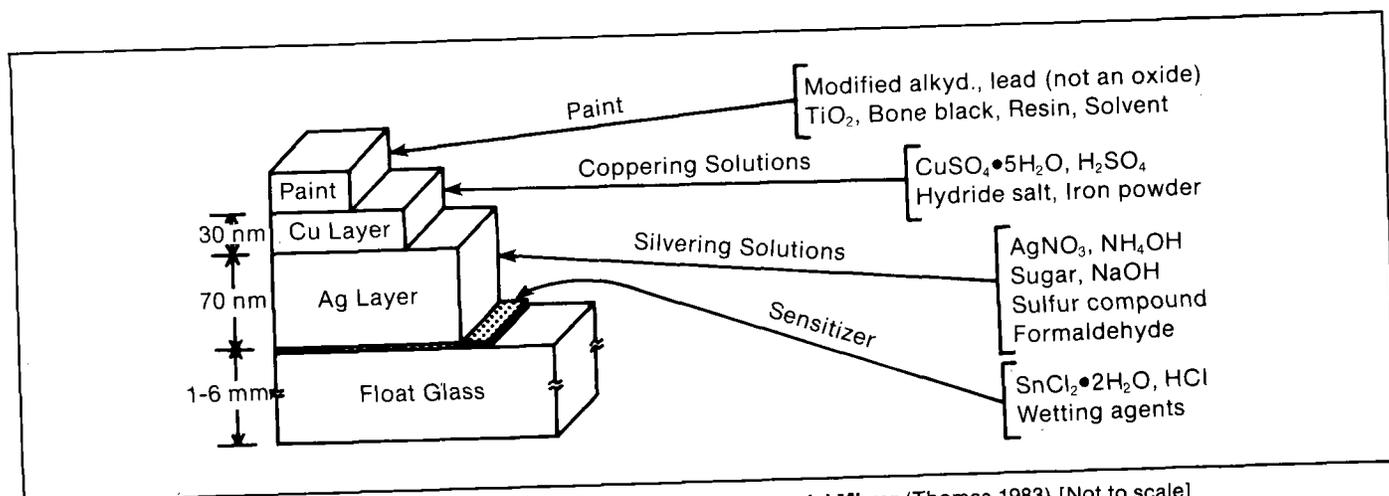
Figure 3-1 Morphology and Chemical Components Used in a Typical Commercial Mirror (Thomas 1983) [Not to scale]
