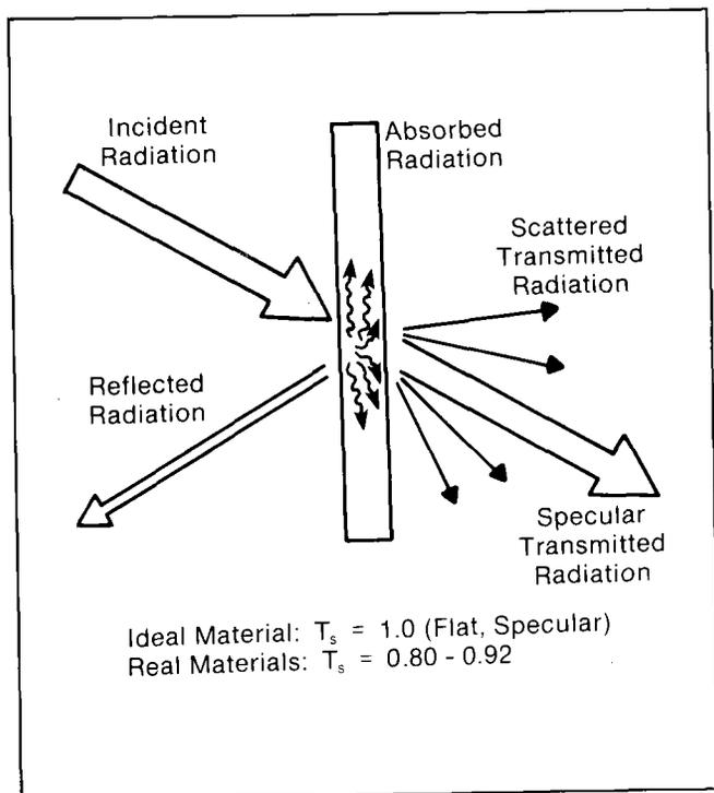
Figure 2-1 Optical Properties of Transmitters (Lind 1981)
