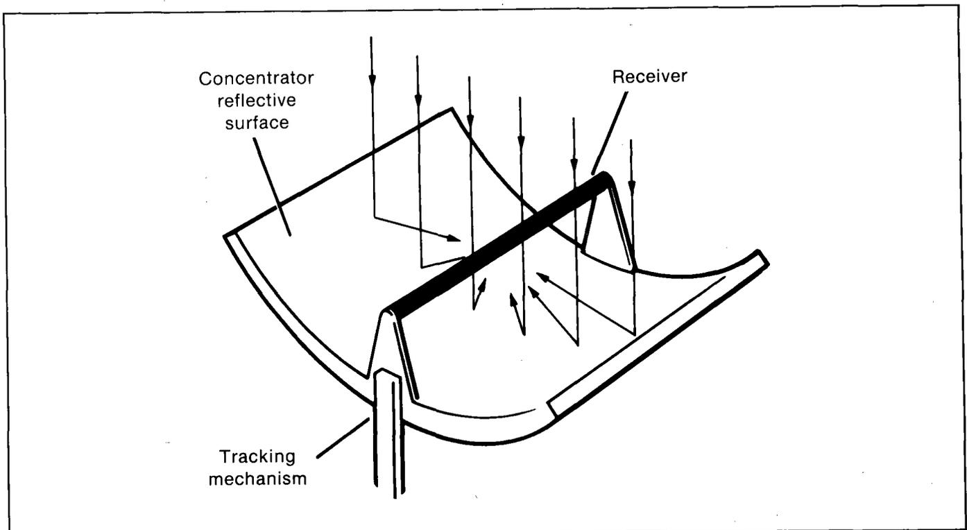
Figure 1-1 Parabolic Trough
