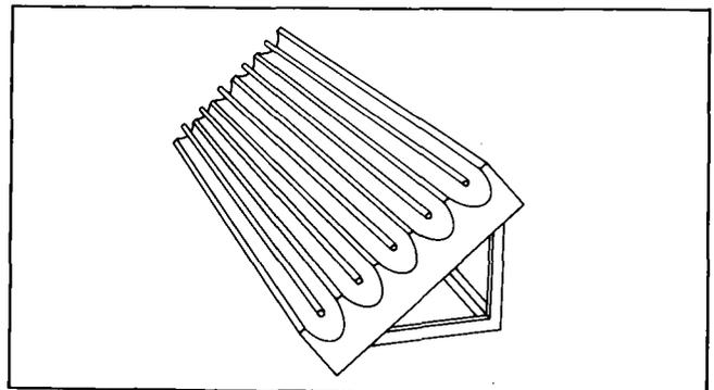
Figure 1-4 Compound Parabolic Concentrator
