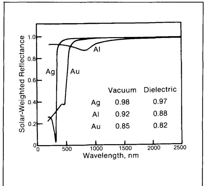
**Figure 2-11 Reflectance Properties of Silver (Ag), Aluminum (Al), and Gold (Au) as a Function of Wavelength for the Metal/Vacuum Interface.** The table lists the solar-weighted reflectance for a metal/vacuum interface and a metal/dielectric interface with an assumed index of refraction of 1.5. (Pettit and Roth 1980)
