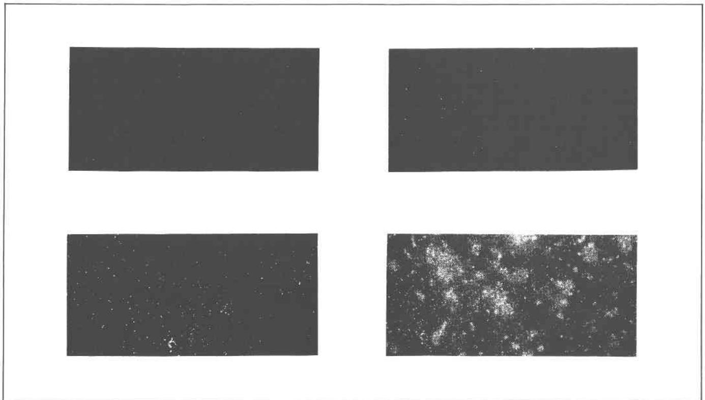
**Figure 4-1 Darkfield Photomicrographs (100x) of Degraded Commercial Mirror** [The exposure periods are as follows: (top, left) unexposed; (top right) after two weeks; (bottom left) after four weeks; (bottom right) after eight weeks.] (Masterson 1983b)
