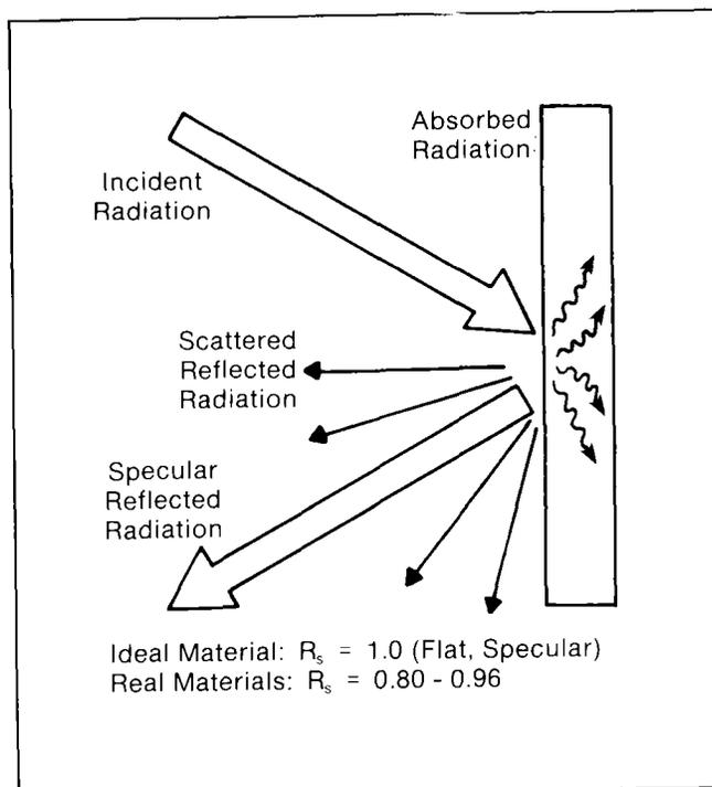
Figure 2-2 Optical Properties of Reflectors (Lind 1981)
