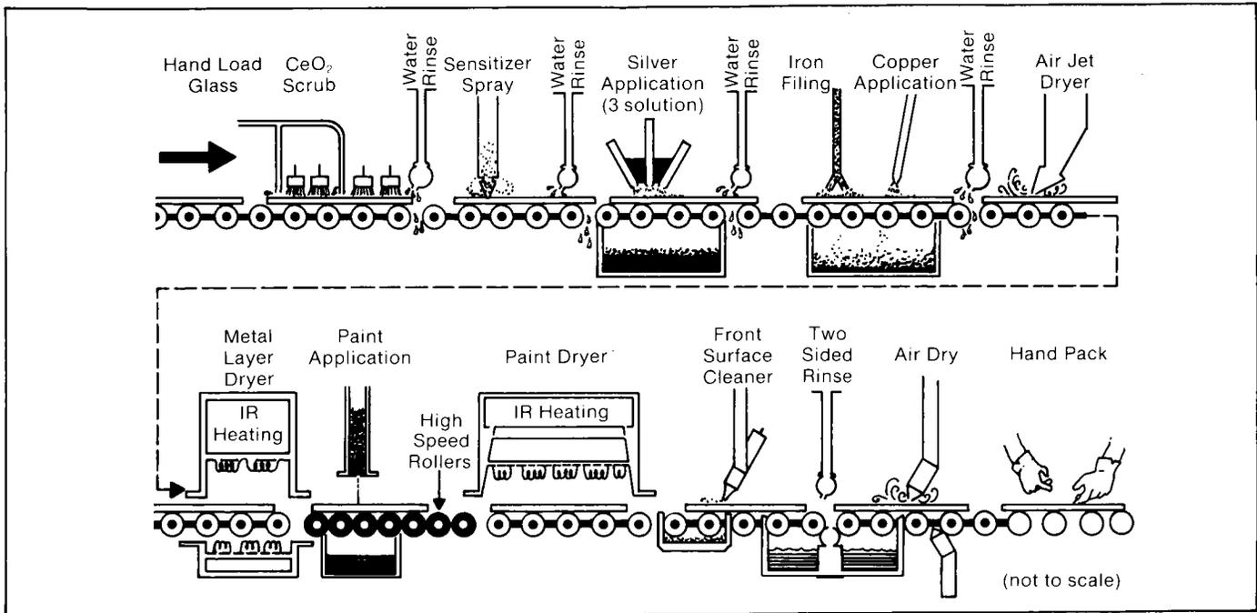
Figure 5-2 Wet-Chemistry Mirror Production Sequence (Lind et al. 1979)
