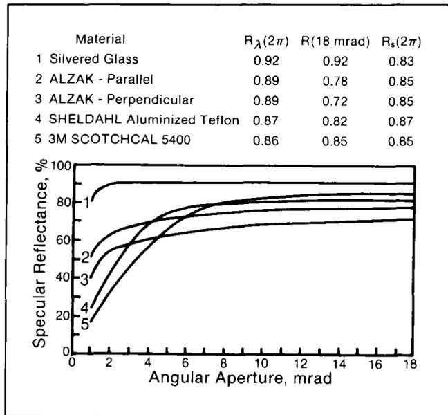
**Figure 2-10 Specular Reflectance Properties for Several Solar Mirror Materials.** The table lists the hemispherical reflectance  $[R_\lambda(2\pi)]$  and the specular reflectance at 18 mrad  $[R(18 \text{ mrad})]$  measured at 500 nm. Also listed is the solar-weighted hemispherical reflectance  $[R_s(2\pi)]$  (Pettit and Roth 1980)
