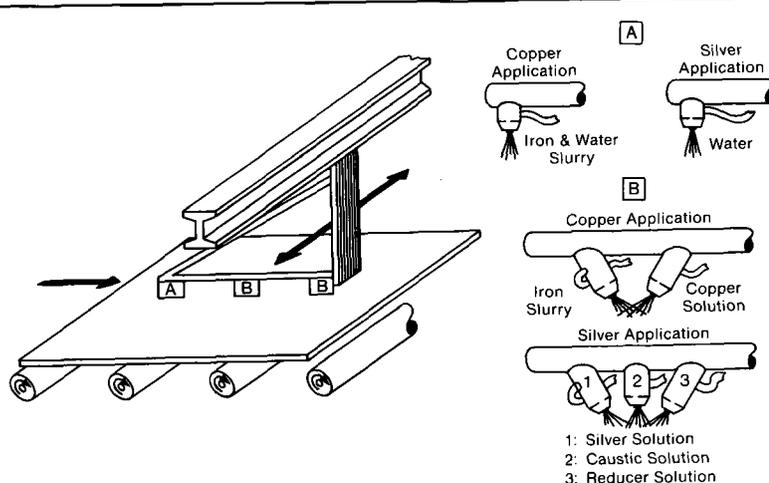
**Figure 5-5 Reciprocating Spray Chemical-Applicator for Wet-Chemistry Mirroring Solutions.** Specific nozzle arrangements are shown for a galvanic copper and a three-part silver process. The details A and B (on right) represent the nozzles placed at A and B on left of illustration. (Lind et al. 1979)
