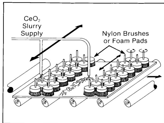
**Figure 5-3 Abrasive Glass-Scrubber Using Continuous Slurry Application and Oscillating Assemblies of Rotating Brushes** (Lind et al. 1979)
