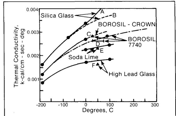
Figure 2-8 Thermal Conductivity of Glasses (Bouquet 1979)
