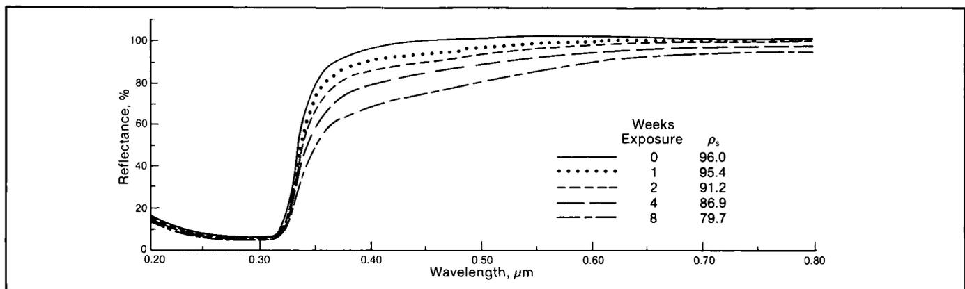
Figure 4-3 Spectral Hemispherical Reflectance for Different Exposures of a Commercial Mirror [Values for the exposure periods and the solar-weighted reflectance ( $\rho_s$ ) are shown in the legend.] (Masterson and Lind 1983a)
