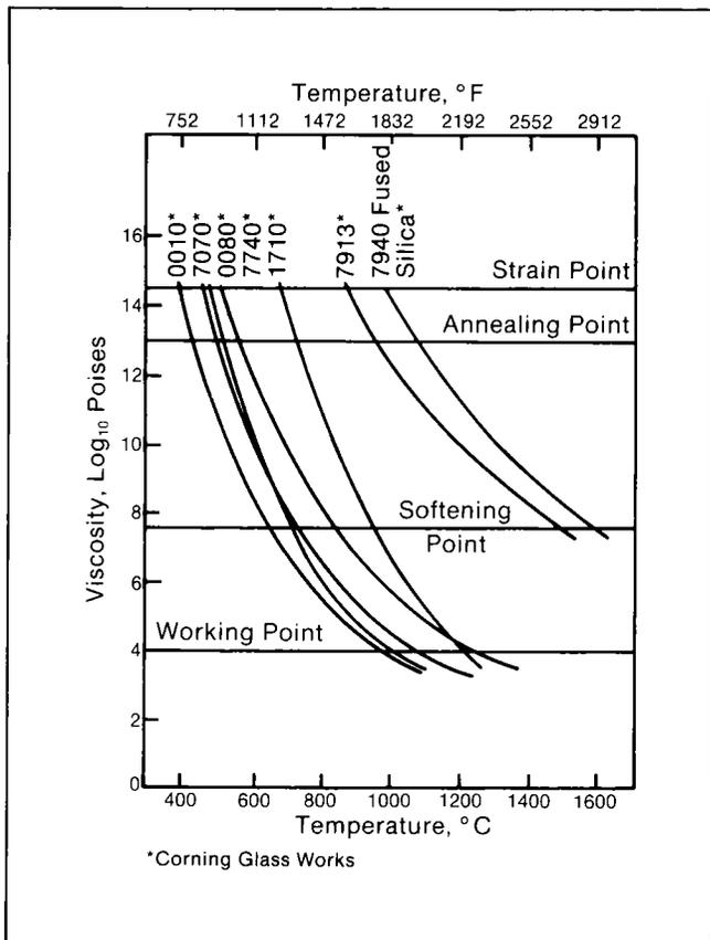
Figure 2-4 Viscosity - Temperature Curves (CIT 1978)
