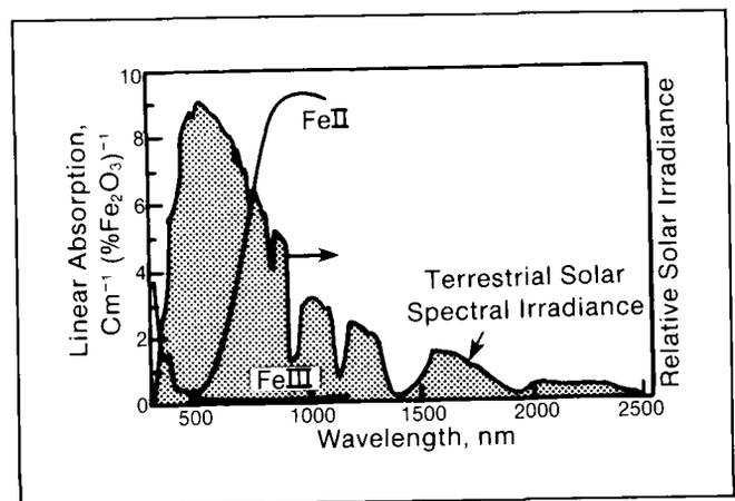
**Figure 2-14 Absorption Coefficients of Fe<sup>+2</sup> and Fe<sup>+3</sup> in Soda-Lime Glass** (The shaded curve is the relative spectral solar irradiance) (Coyle 1981)
