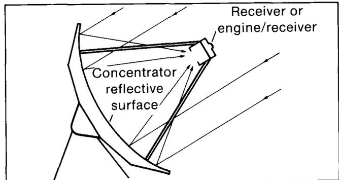
Figure 1-2 Parabolic Dish
