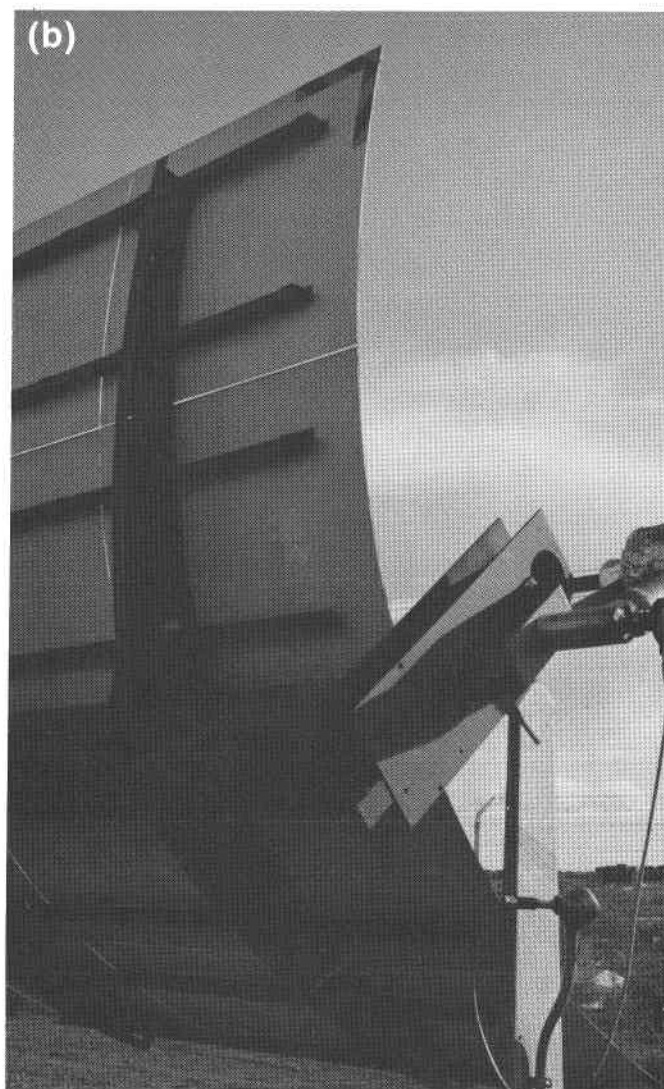
Figure 2.3. A Stamped Ribbed Sheet Metal Parabolic Trough (a) and a Sagged Glass Parabolic Trough (b)
