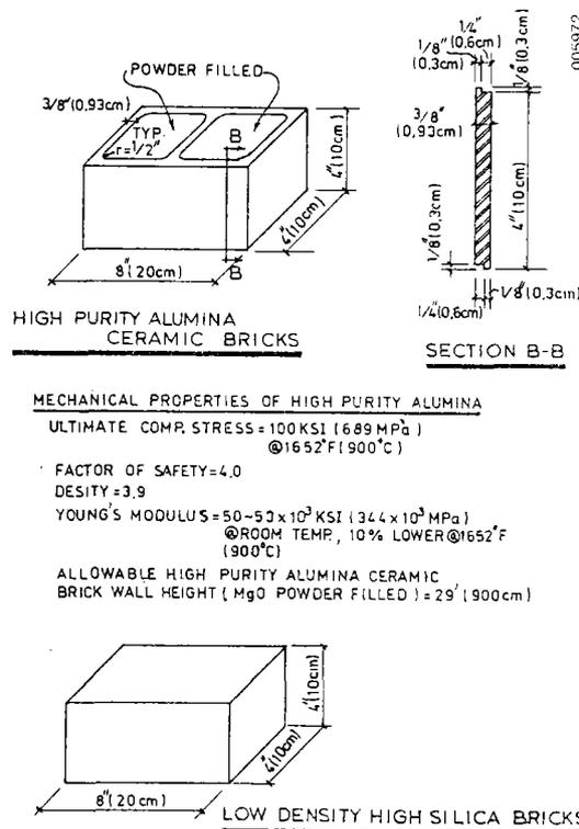
Figure 5-10. Details of Ceramic Bricks Used in Figure 5-7
