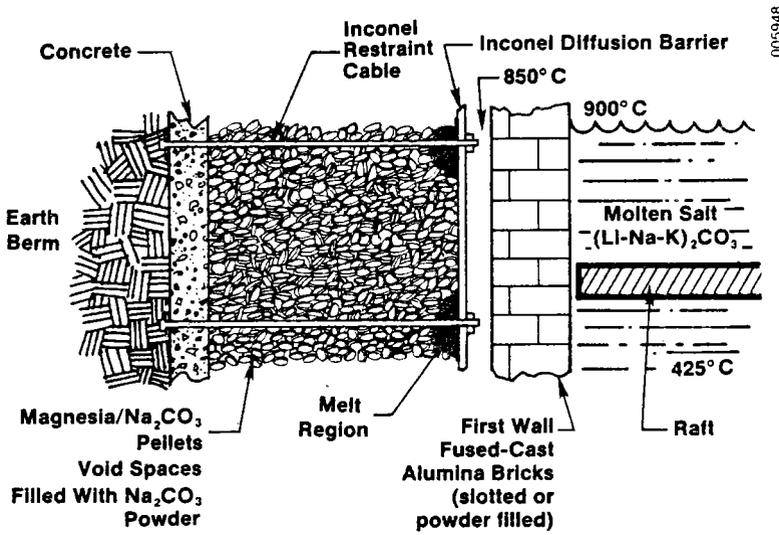
Figure 2-4. Single-Tank Raft Thermocline System with Alumina Bricks and Pellet Insulation
