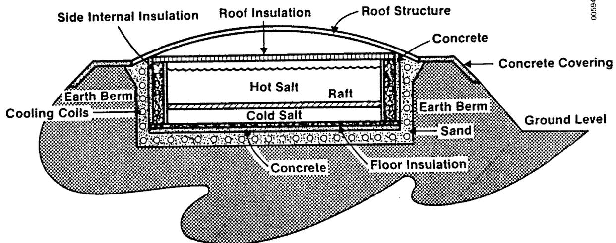
Figure 2-1. Single-Tank Raft Thermocline Storage Concept
