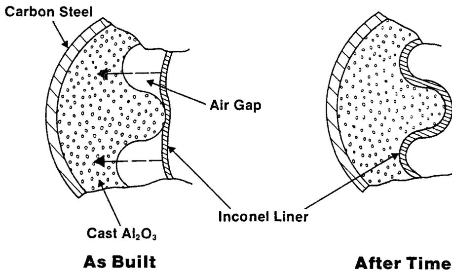
Figure 2-17. Detail of Inconel Liner for Two-Tank Storage Shown in Figure 2-16
