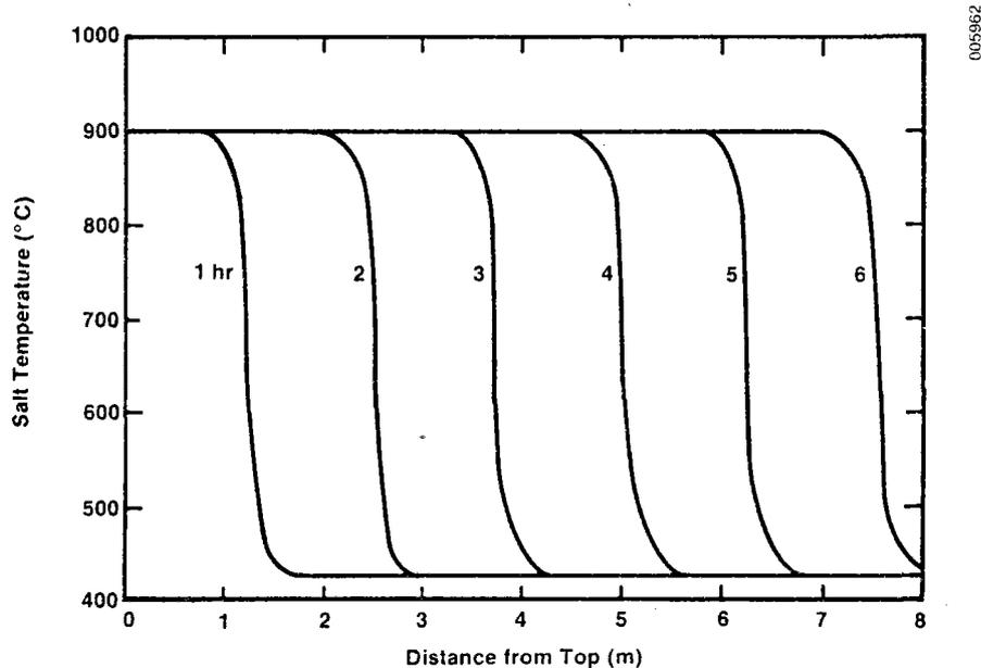
Figure 4-1. Molten Salt Temperature Distribution In A Packed Magnesia-Pellet Bed. Void Fraction = 30%, Pellet Diameter = 2.54 cm., Fluid Superficial Velocity = 0.03 cm/sec.
