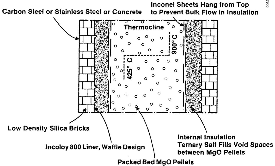
Figure 2-7. Single-Tank, Two-Media, Thermocline System--Cylindrical Storage Tank
