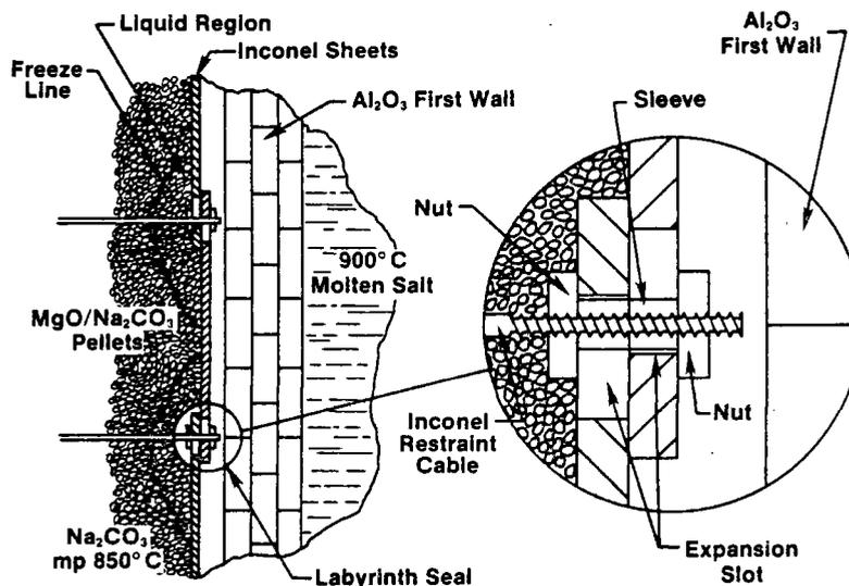
Figure 2-5. Details of Diffusion Barrier Shown in Figure 2-4
