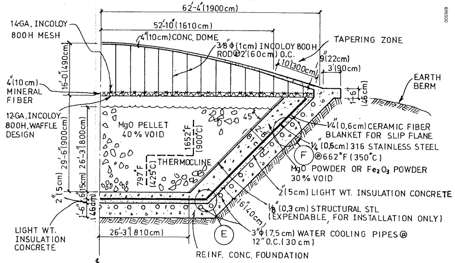
Figure 5-7. Details of Single-Tank, Two-Media, Sloped-Wall Tank (Reinforced Concrete Tank). Also refer to Figure 2-8
