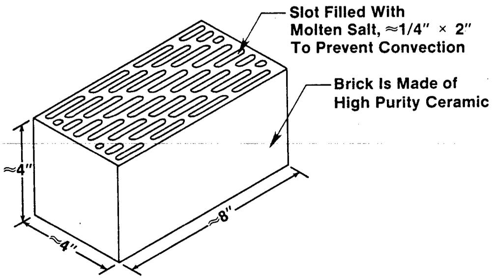
Figure 2-3. Slotted High-Purity Alumina Brick
