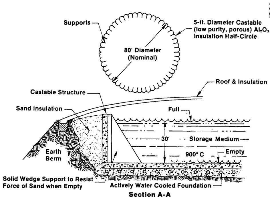
Figure 2-12. Two-Tank System with Unlined Castable Structure
