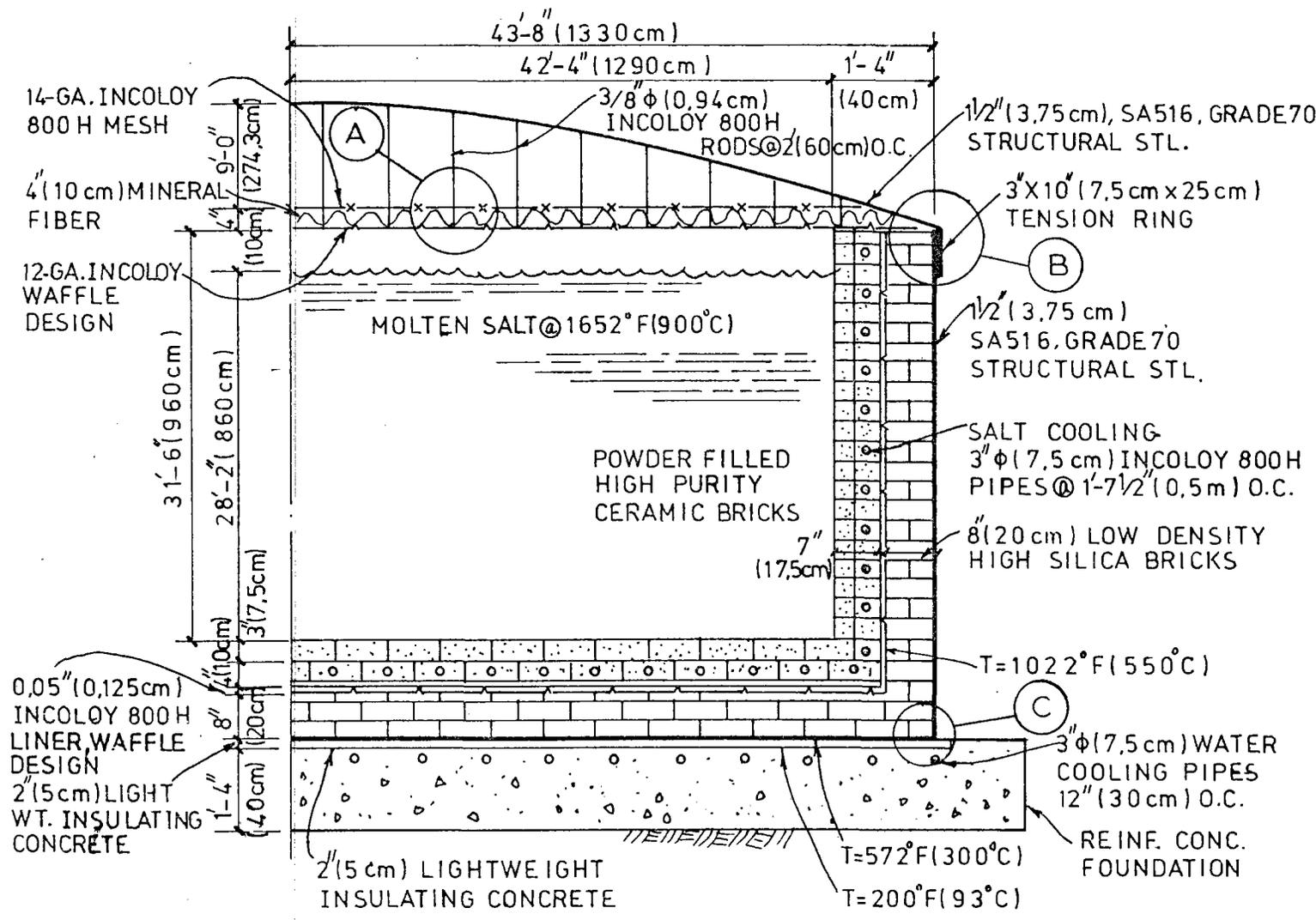
Figure 5-9. Details of Two-Tank System with Multiple-Layered Insulation and Actively Cooled Hot Tank (Steel Tank). Also refer to Figure 2-10
