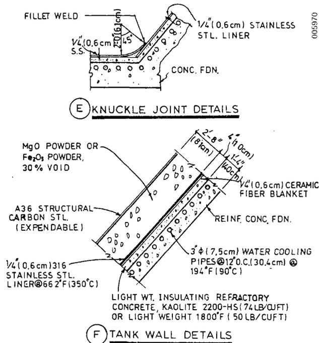
Figure 5-8. Details of Several Cross-Sections in Figure 5-7
