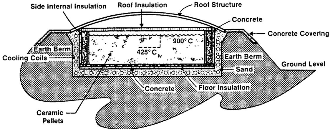
Figure 2-6. Single-Tank, Two-Media, Thermocline Storage Concept
