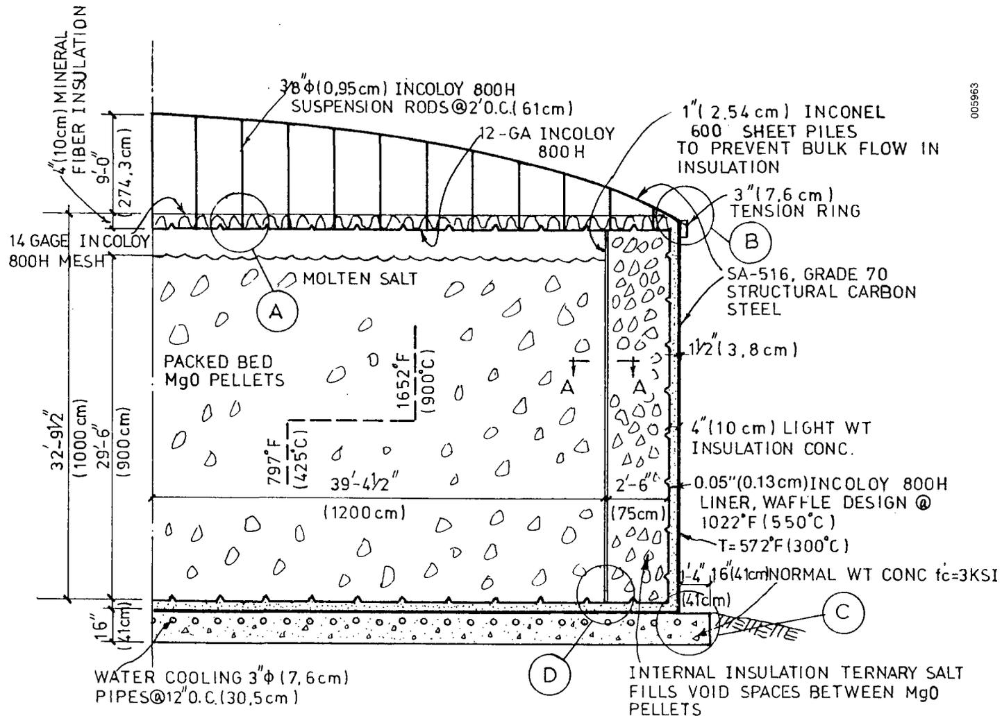
Figure 5-1. Details of Single-Tank, Two-Media Cylindrical Tank (Steel Tank).
