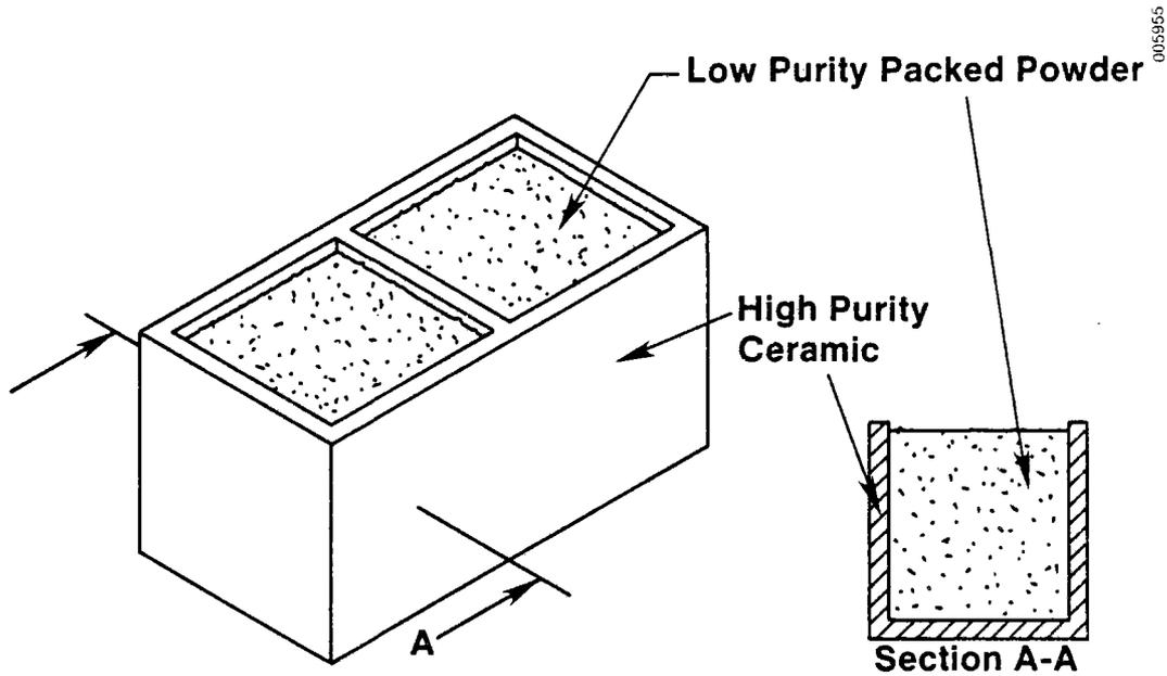
Figure 2-11. Powder-Filled, High-Purity Alumina Brick.
