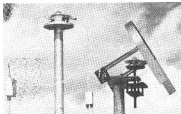
Total Insolation Pyranometer Diffuse Insolation Pyranometer
