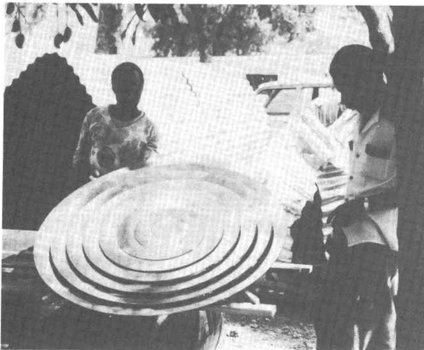
Figure 10. Completed Spiral Concentrator
