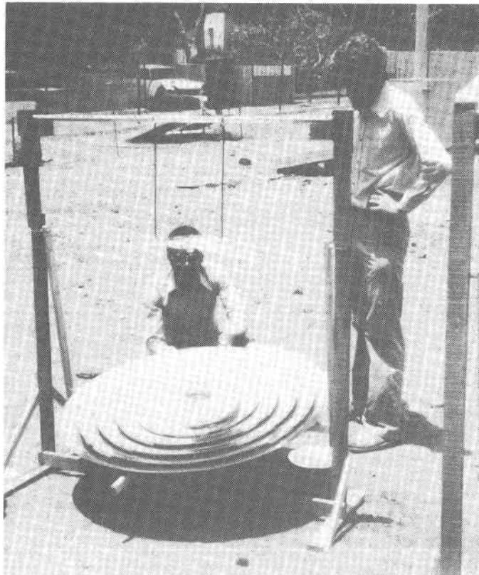
Figure 14. The Spiral Concentrator Igniting Wood at the Focal Point
