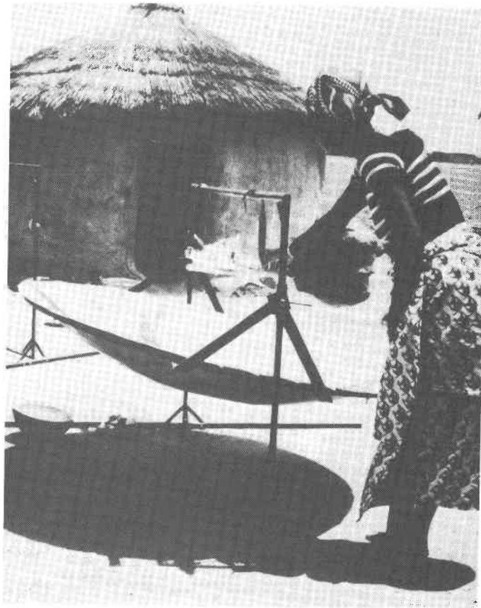
Figure 2. Solar Cooker Used in Danchurchaid Program in Upper Volta
