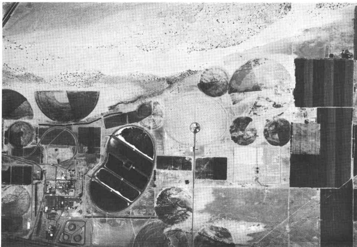
Figure 2.5. Aerial photograph of the Solar One site and vicinity in June 1984. The rectangular light area to the lower right of the heliostat field is an array of parabolic troughs. The circular and pie-shaped sectors are agricultural plots begun in the winter of 1983. The dark and light banded rectangles to the right are agricultural fields bordering the Coolwater property. The dry Mojave River bed runs across the top of the photo.
