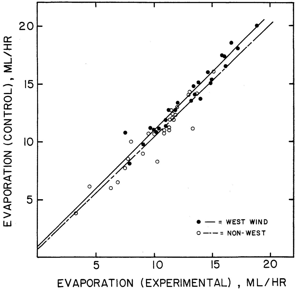
Figure 4.9 Evaporation rates measured at a control site plotted against those measured simultaneously downwind of the Solar One heliostat field.
