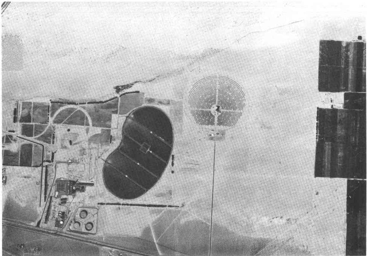
Figure 2.4. Aerial photograph of the Solar One site and vicinity on March 1982 just prior to dedication of the completed facility. The circular track left center is a coal gasification combined cycle facility under construction. Coolwater units 1, 2, 3 and 4 are lower left. Dark squares and rectangles are agricultural crop land. The dry Mojave River bed cuts diagonally across the top of the photo.
