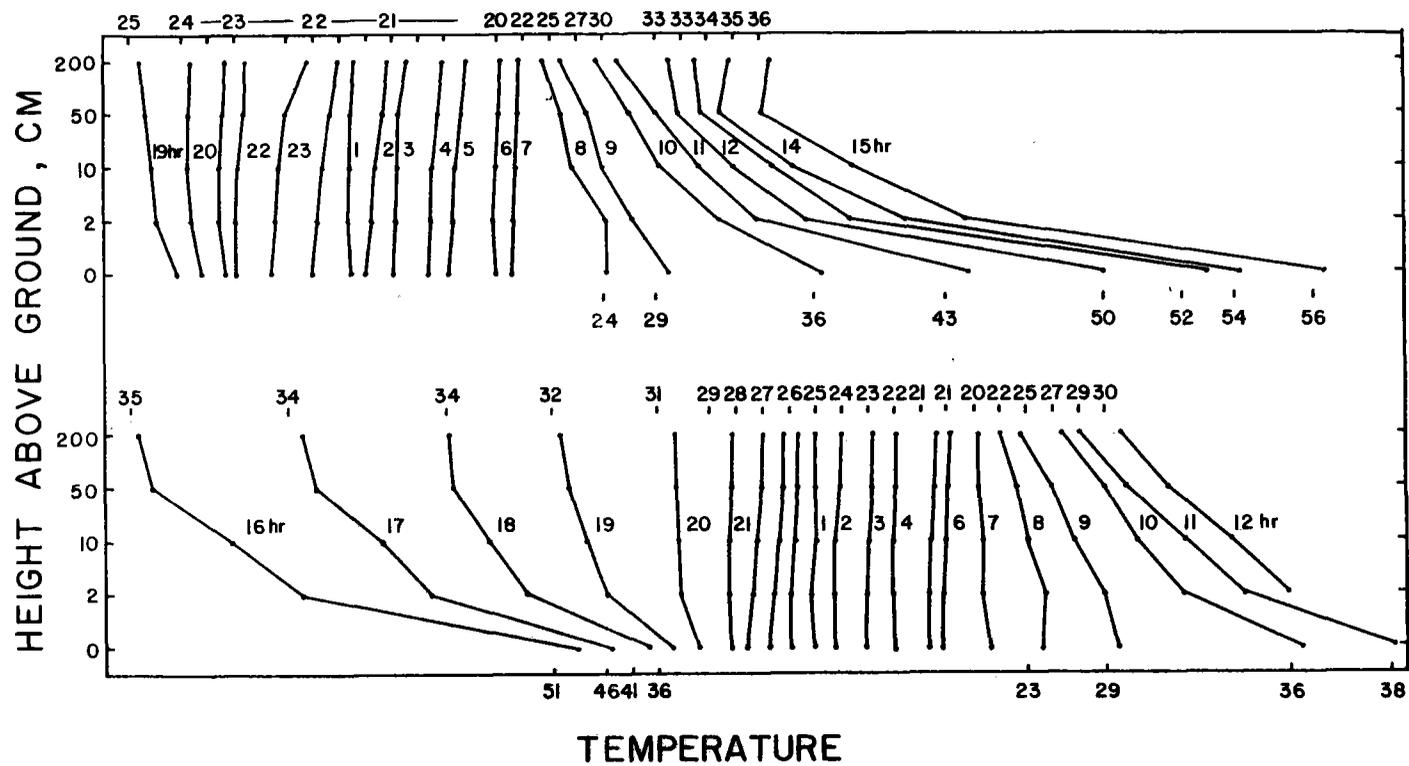
Figure 4.7 Air temperature profiles measured outside of the Solar One heliostat field over a 41-h period between 1900 h August 27 and 1200 h August 29, 1982.
