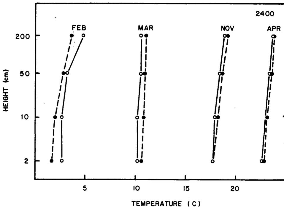
Figure 4.2 Air temperature profiles (at 2400 hours) at two sites near the heliostat field between November 1980 and April 1981. Symbols as in Figure 4.1.
