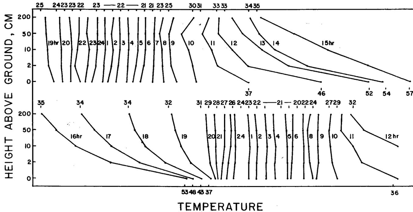
Figure 4.6 Air temperature profiles measured within the Solar One heliostat field over a 41-h period between 1900 h August 27 and 1200 h August 29, 1982.
