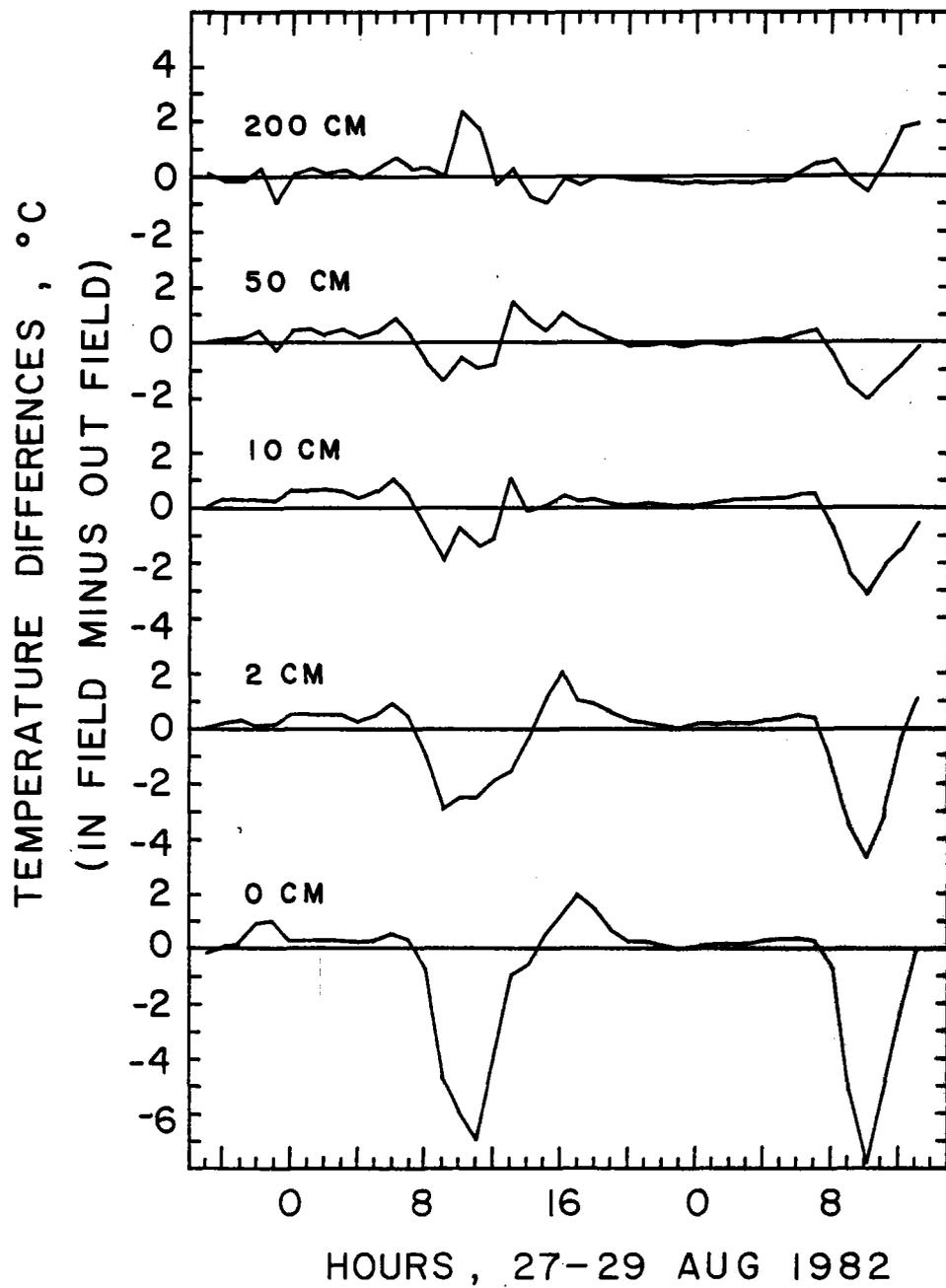
Figure 4.5 Differences in air temperatures measured within the Solar One heliostat field and 25 m outside of the heliostat array in August 1982.
