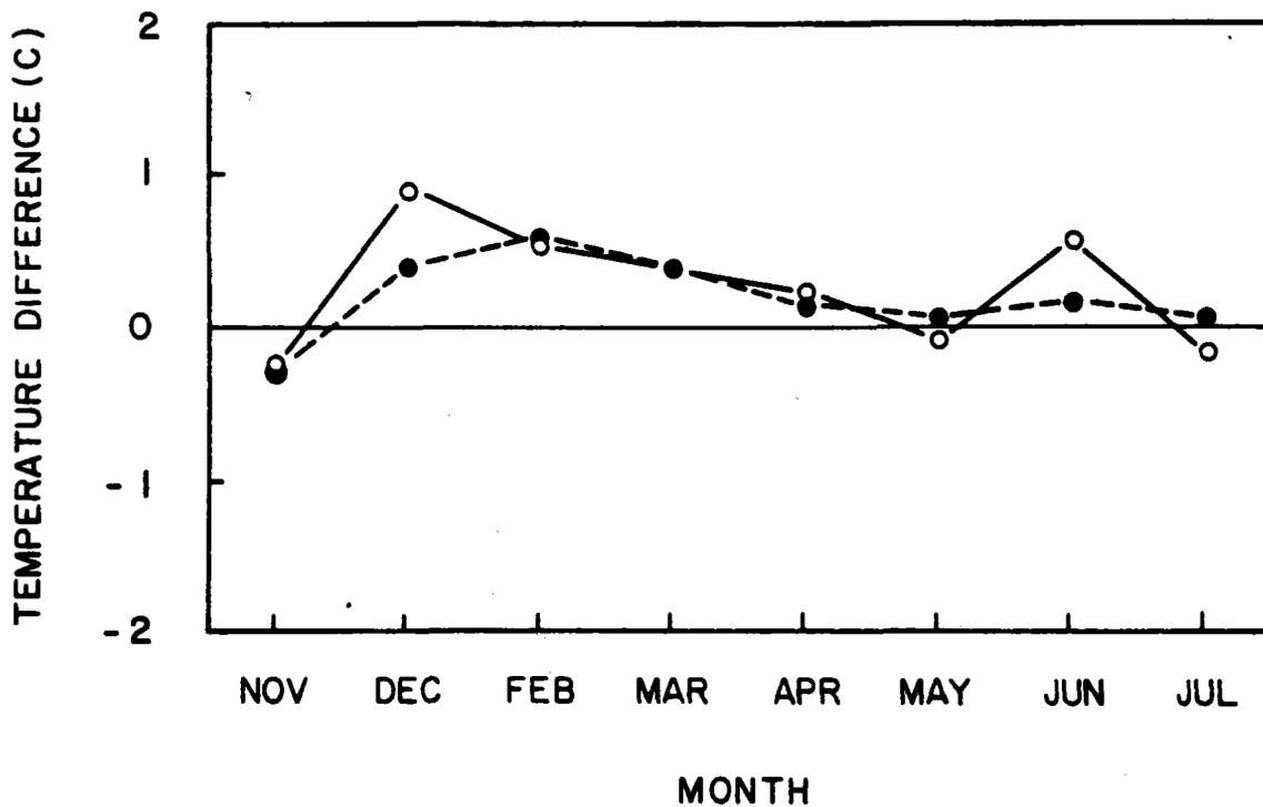
Figure 4.4 Differences between mean temperatures (at 2 m) at two sites near the heliostat field between November 1980 and July 1981. Open circles: mean nighttime minimum temperature differences; solid circles: mean nighttime temperature differences.
