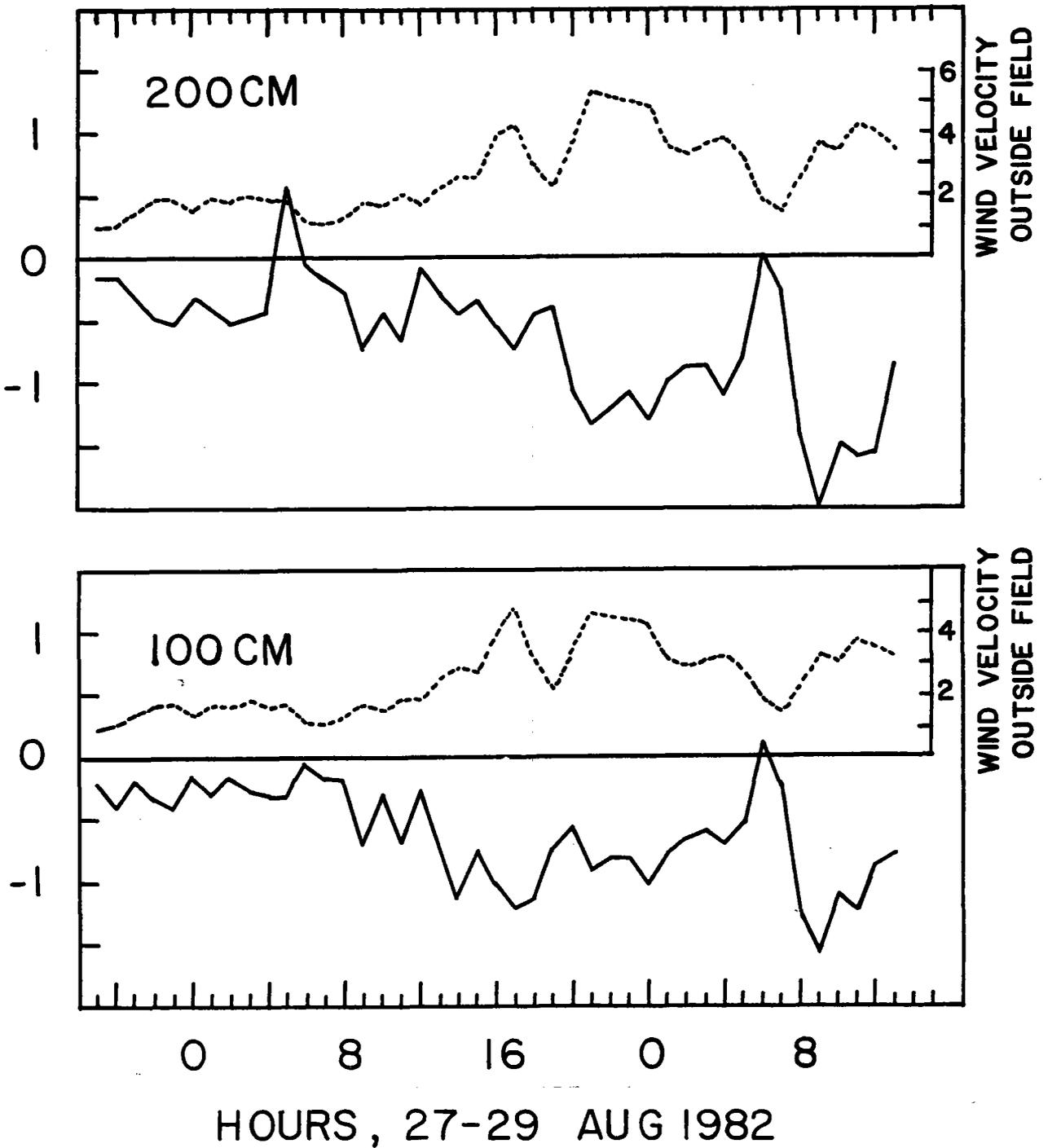
Figure 4.10 Wind speeds measured outside the Solar One heliostat field (above) and differences between wind speeds measured within and outside the heliostat array (below).
