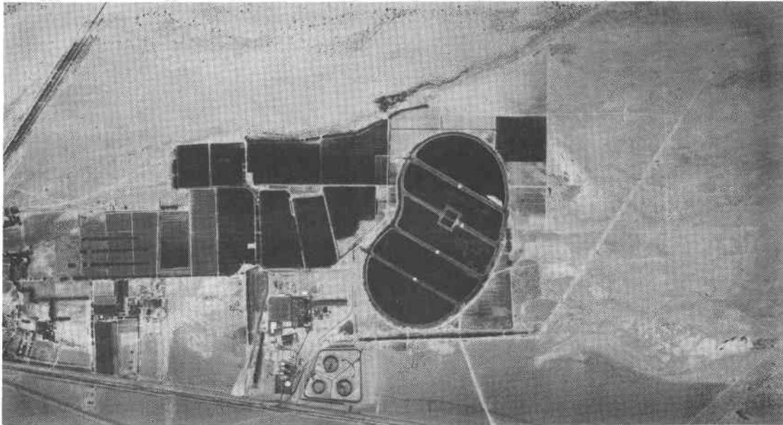
Figure 2.2A. Southern California Edison's Coolwater Generating Station (left center) in July 1979. Large kidney-shaped area is composed of evaporating ponds. Dark rectangular areas are agricultural fields. The site of the prospective solar thermal power plant is in right center.
