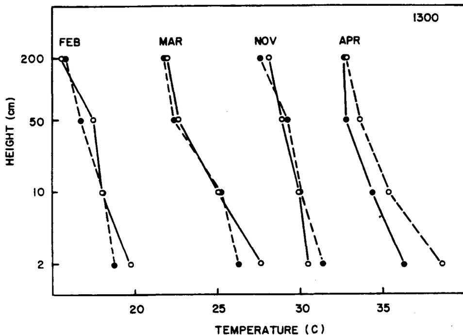
Figure 4.1 Air temperature profiles (at 1300 hours) at two sites near the heliostat field between November 1980 and April 1981. Open circles: experimental site (directly downwind of the heliostat field); solid circles: control site.
