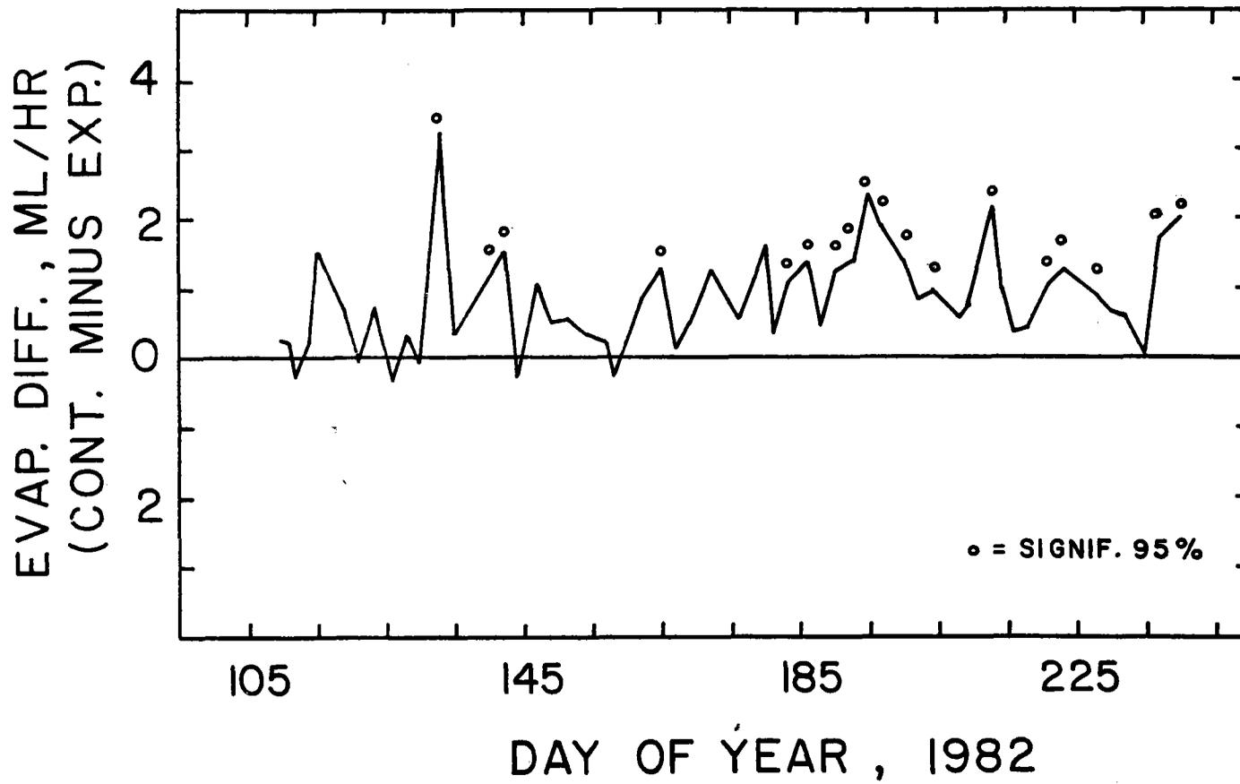
Figure 4.8 Differences in evaporation rates measured at a control site and at a point 25 m downwind of the Solar One heliostat field in 1982.
