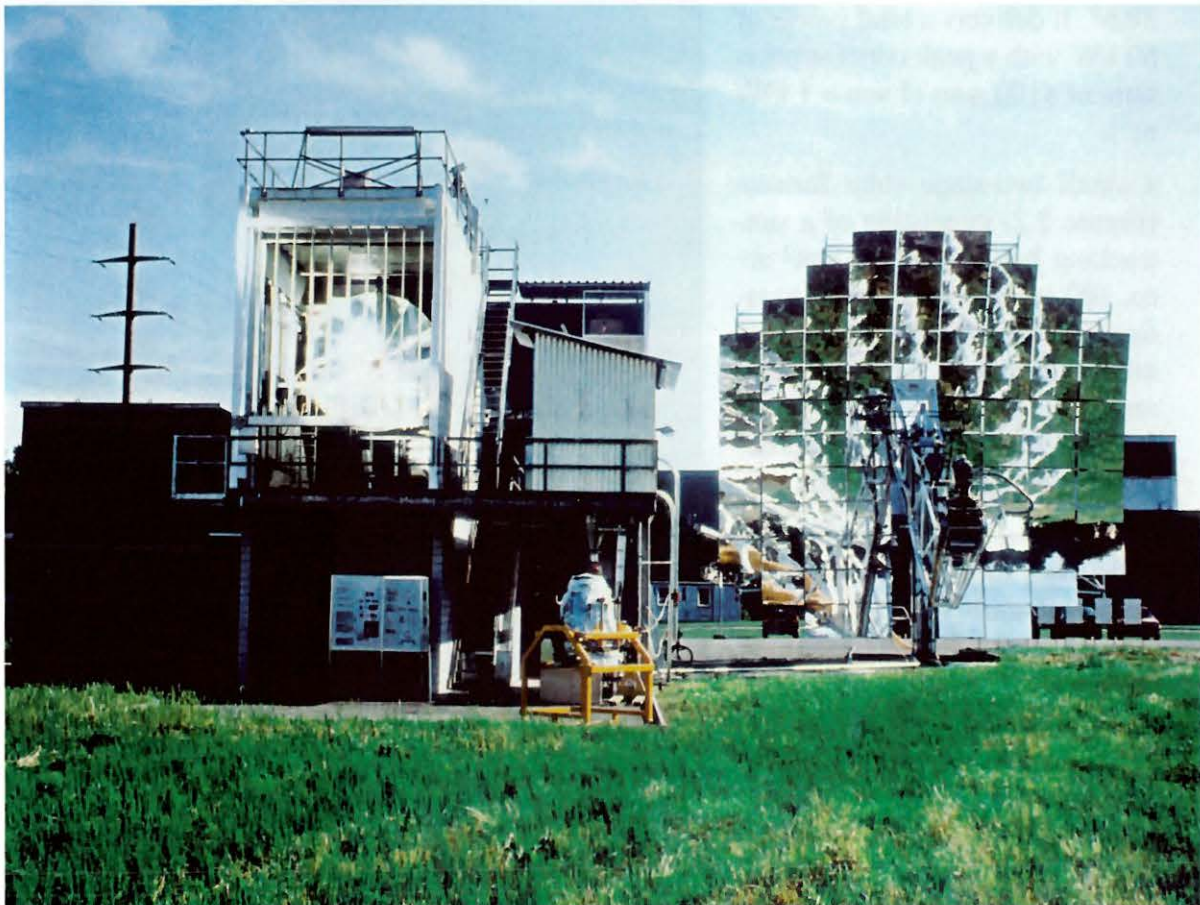
Figure 2.2 PSI 's 15 kW solar furnace (left) and 60 kW parabolic concentrator (right)
