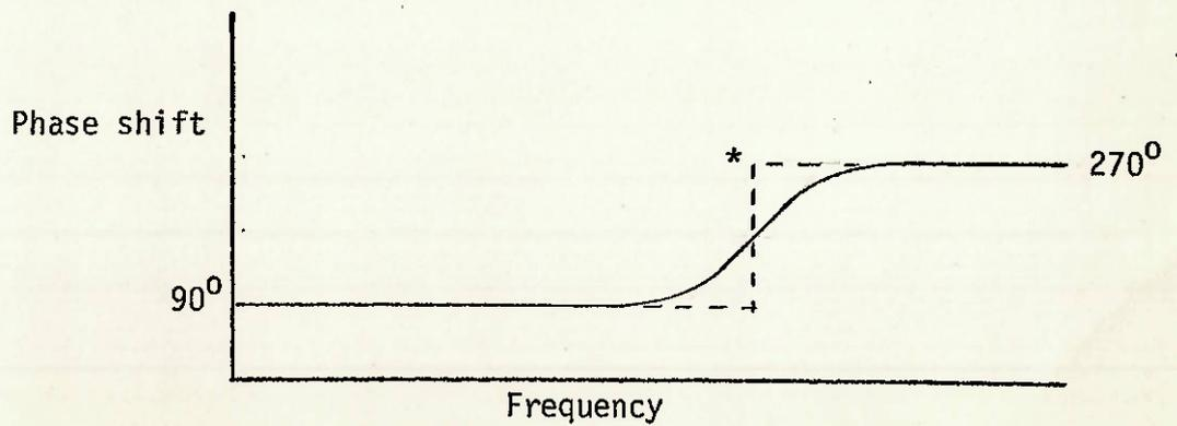
\* Dashed lines indicate position of resonance (if damping were negligible)
