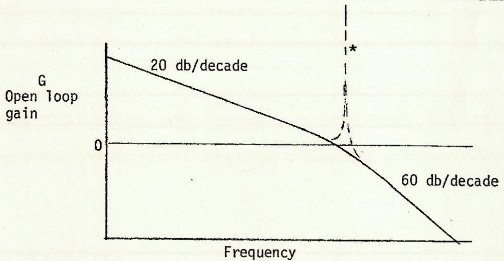
FIGURE 3: Gain and phase vs frequency
